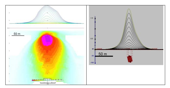
Figure F-3: Maxwell plate model and RDI from the calculated response for bulk ("thick") 100 m length, 40 m depth extend, 30 m thickness
