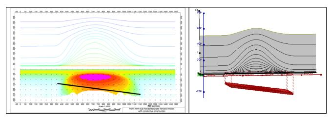
Figure F-8: Maxwell plate model and RDI from the calculated response for the long, wide and deep subhorizontal plate (depth 140 m, dim 25x500x800 m) with conductive overburden.
