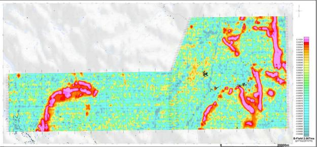
VTEM B-Field Z Component Channel 38, Time Gate 2.667 ms
