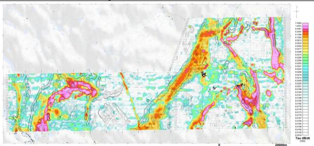
dB/dt Calculated Time Constant (Tau) with contours of anomaly areas of the Calculated Vertical Derivative of TMI
