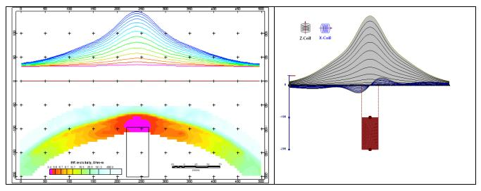
Figure F-4: Maxwell plate model and RDI from the calculated response for "thick" vertical target (depth 100 m, depth extend 100 m). 19-44 chan.
