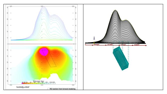
Figure F-7: Maxwell plate model and RDI from the calculated response for inclined thick (50m) plate. Depth extends 150 m, depth to the target 50 m.
