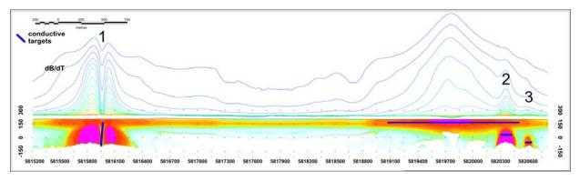
Figure E-4: dB/dt profile and RDI with different depths of targets.
