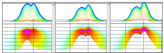
Figure F-9: Maxwell plate models and RDIs from the calculated response for "thick" dipping plates (35, 50, 75 m thickness), depth 50 m, conductivity 2.5 S/m.
