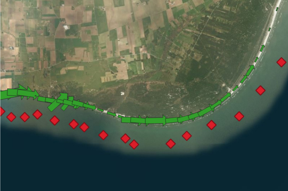
Figure 13. The results for the longshore sediment transport estimates at Sandhammaren. The green arrows indicate the modeled direction and magnitude of the net transport. The red dots indicate the wave model grid nodes where the wave information was extracted for the longshore sediment transport estimates. The colored background represents the bathymetry scaled from green (shallow) to red (deep).
