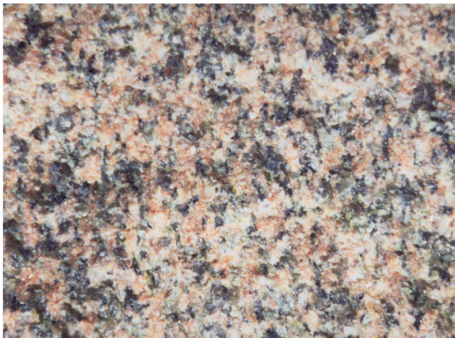
Fig. 2. Photograph of Vätö granite. The feldspar megacrysts are on average 12 mm long.
