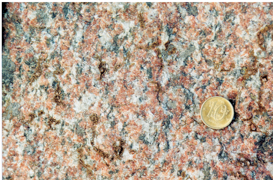
Fig. 2. Medium-grained Småland granite from sample locality KK 94:33, Vägghytan. (The diameter of the coin is 20 mm.)
