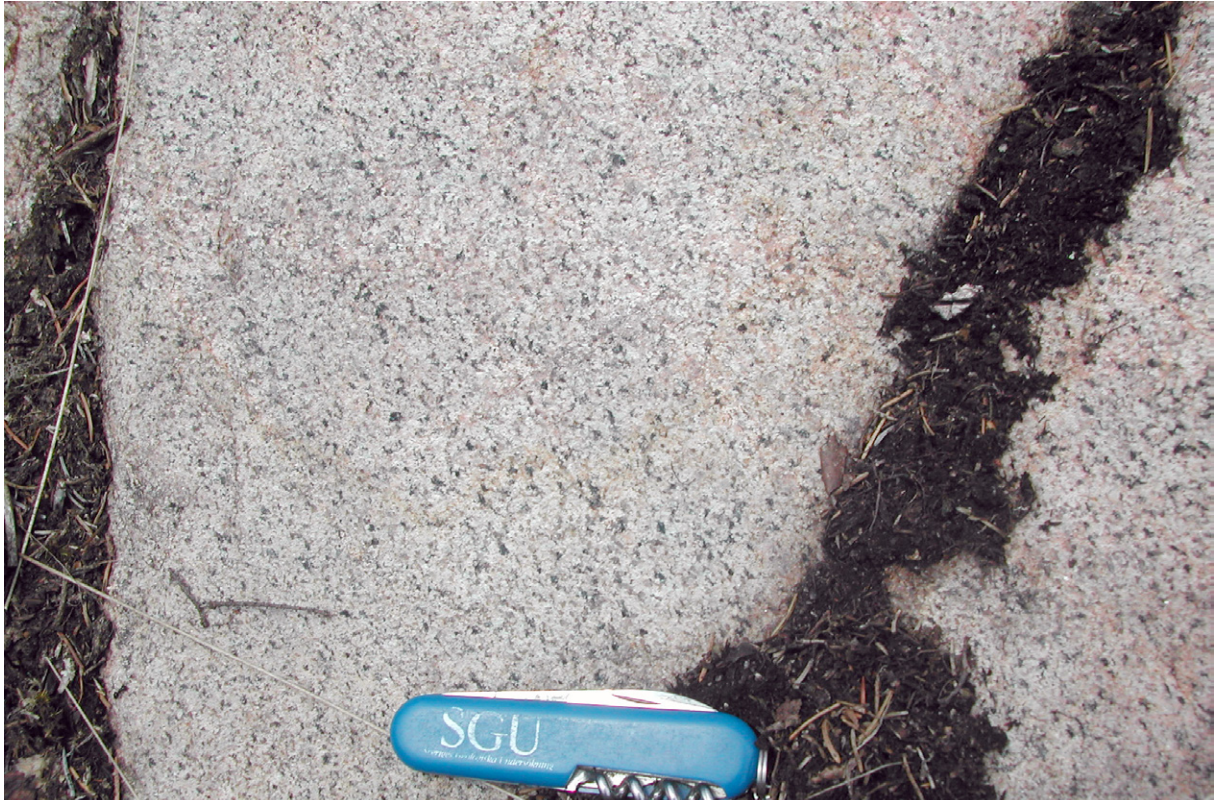
Fig. 45. Jämnkornig monzogranit, 4D Markaryd SO (o g), 6252789/1382039. Foto: Ulf Bergström. Even-grained monzogranite.
