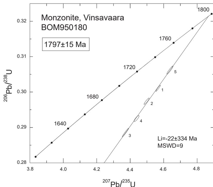
Figure 5. Concordia diagram for analysed zircon fractions from the monzodiorite sample BOM950180, Vinsavaara.
