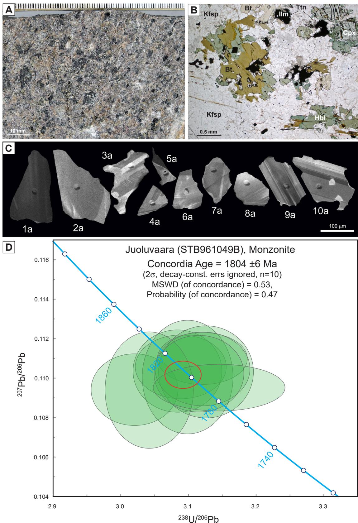
Figure 6. Geochronology of the Juoluvaara monzonite. **A.** The dated rock sample. **B.** Photomicrograph of dated sample. **C.** Cathodoluminescence (CL) images of analysed zircon grains. Numbers refer to analytical spot number in Table 3. **D.** Tera Wasserburg diagram showing U-Pb SIMS data of analysed zircon from monzonite sample STB991049B, Juoluvaara. Error ellipse of calculated weighted mean age is shown in red. All photographs by Fredrik Hellström.
