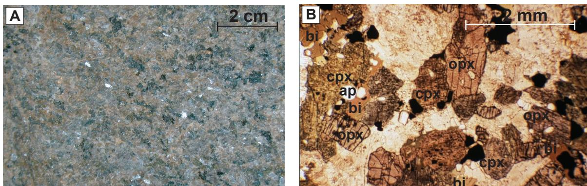
Figure 2. The Vinsavaara monzodiorite. **A.** Photograph of analysed sample. **B.** Photomicrograph of analysed sample showing orthopyroxene, clinopyroxene, biotite and apatite in a matrix of perthitic feldspar. opx - orthopyroxene, cpx - clinopyroxene, bi - biotite, ap - apatite. All photographs by Olof Martinsson.
