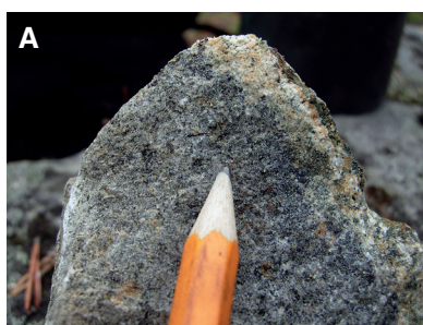
Figure 24. A. Intermediate volcanic rock with a magnetic susceptibility of 0.03 SI. The light area of the rock is the weathered surface. (E 799311, N 7487739, ID: CJO141063).
