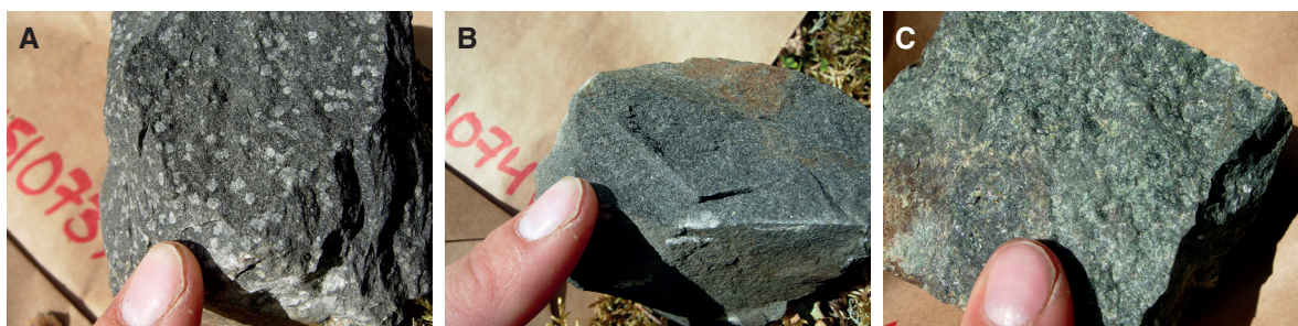
Figure 26. A–C shows different appearances of the basaltic rock intercalated in a sedimentary rock unit. The samples were taken within 10 m of each other (SWEREF99 TM: E 806837, N 7489784. ID: CJO151073).
