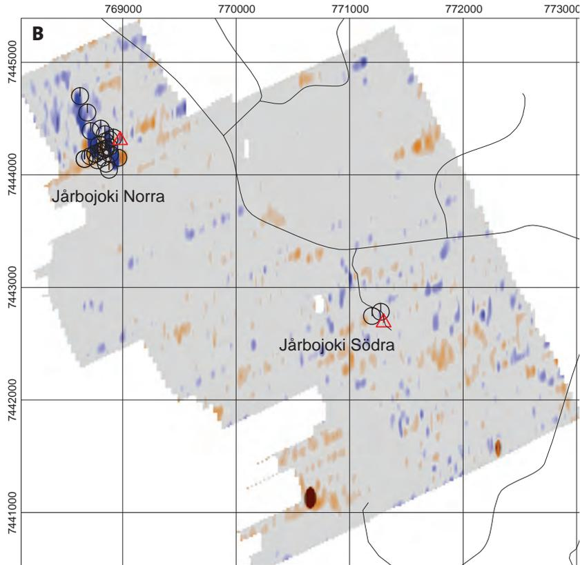
Figure 156. **B.** Electromagnetic (slingram imaginary component) ground measurements of Järbojoki Norra and Järbojoki Södra. Drill hole locations are marked with black circles. Red triangles show the location of sulphide mineralisations.
