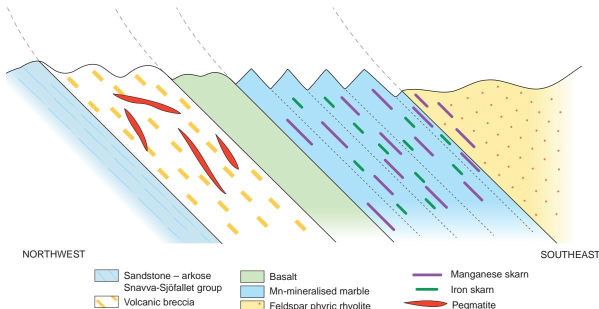
Figure 168. Profile at the Rakten locality. The manganese skarn mineralisation occurring at the contact zone between felsic volcanic rocks of the Arvidsjaur group, and overlying metasedimentary rocks of the Snavva-Sjöfallet group are shown. The stratigraphic sequence is overturned. Illustration: Per Nysten and Tone Gellerstedt.
