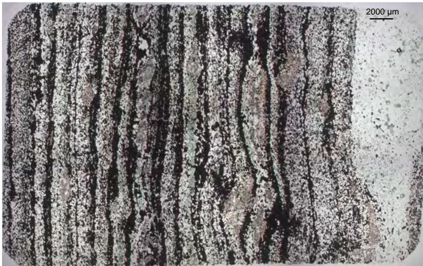
Figure 162. A fine laminated appearance is defined by the distribution of the opaque minerals at Kallak, plane-polarised light. Photomicrograph: Dick Claeson.
