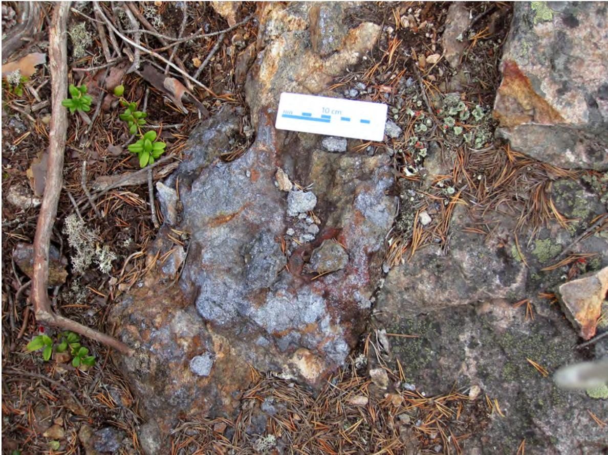
Figure 182. Fracture zone with compact molybdenite in hydrothermally altered granite, rhyolite and pegmatite (7421196/709317). Photo: Ildikó Antal Lundin.
