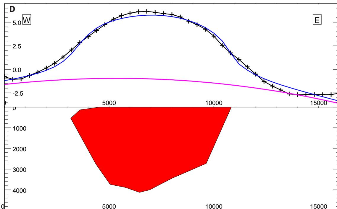
Figure 75. **D.** Modelled profile over the anomaly at Tjaktjajure. Modelled geological body (below) and corresponding geophysical response (above).
