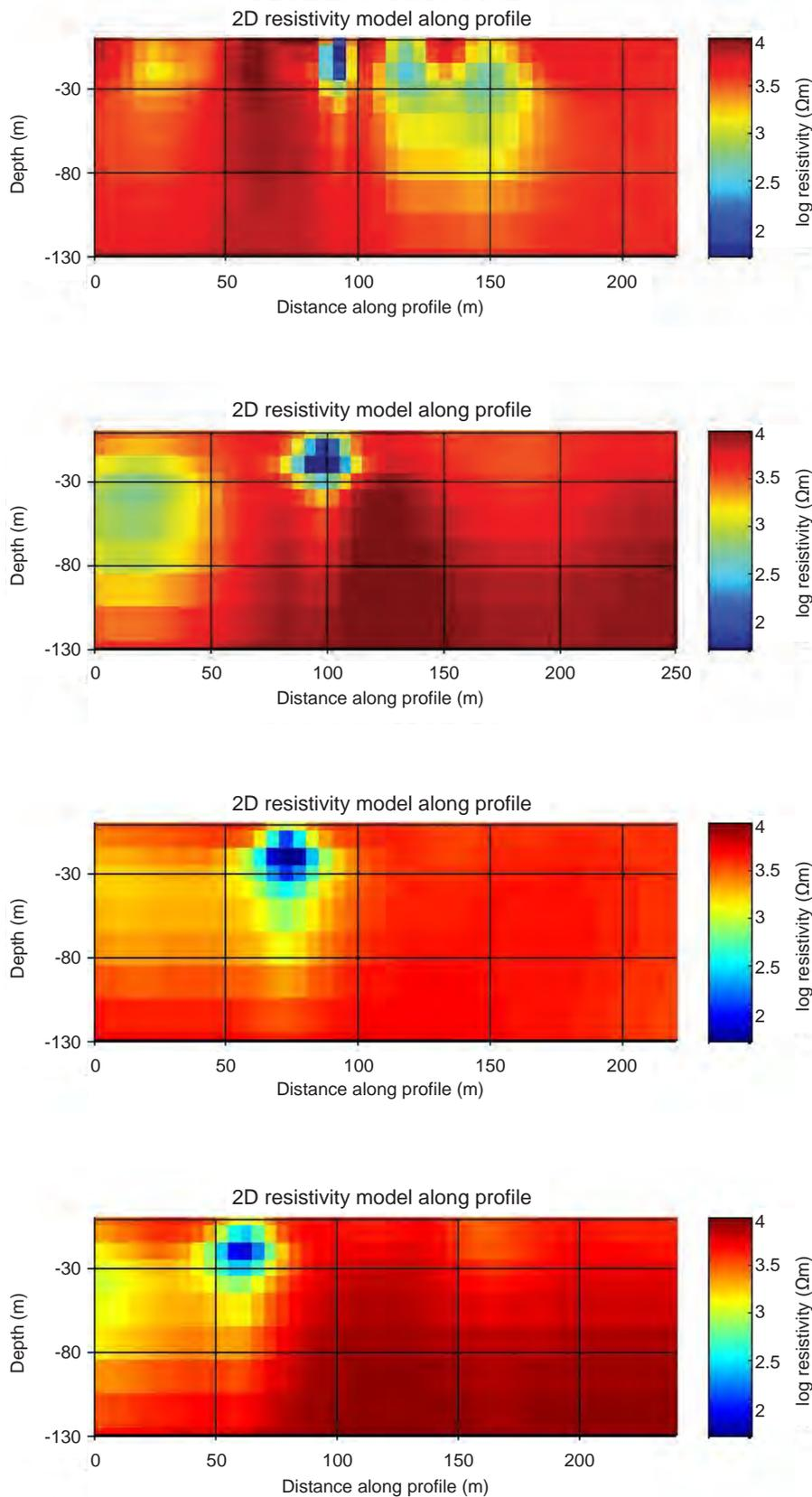
Figure 176. Resistivity models derived from VLF data. The profiles are arranged from north to south, where the first image corresponds to the northernmost profile in Figures 175a–c. The mineralisation indicated shows very low resistivity (dark blue).
