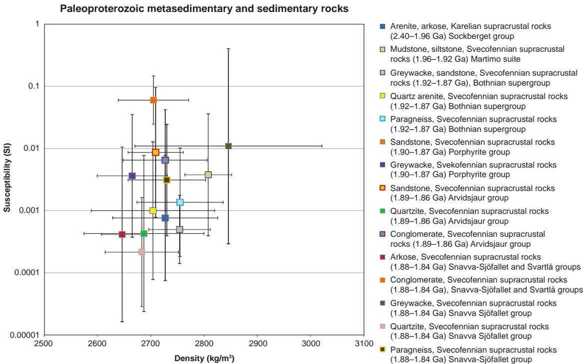
Figure 105. Magnetic susceptibility v. density for Palaeoproterozoic metasedimentary and sedimentary rocks.
