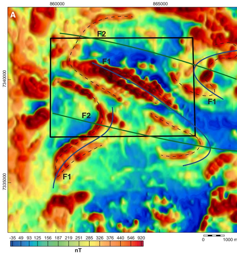
Figure 115. **A.** Fold interference pattern northwest of Kalix interpreted from magnetic anomaly data. Broken black lines are magnetic maxima representing different lithologies within a metasandstone unit, mafic bands within that unit and contacts with felsic meta-intrusive rocks. Blue lines are interpreted  $F_1$  fold axial traces and green lines  $F_2$  axial traces.
