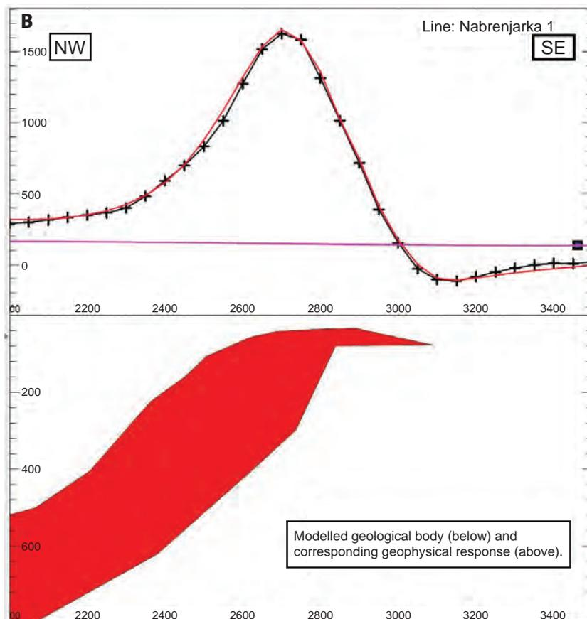
Figure 82. **B.** Geophysical model of the Nabrenjarka dolerite.
