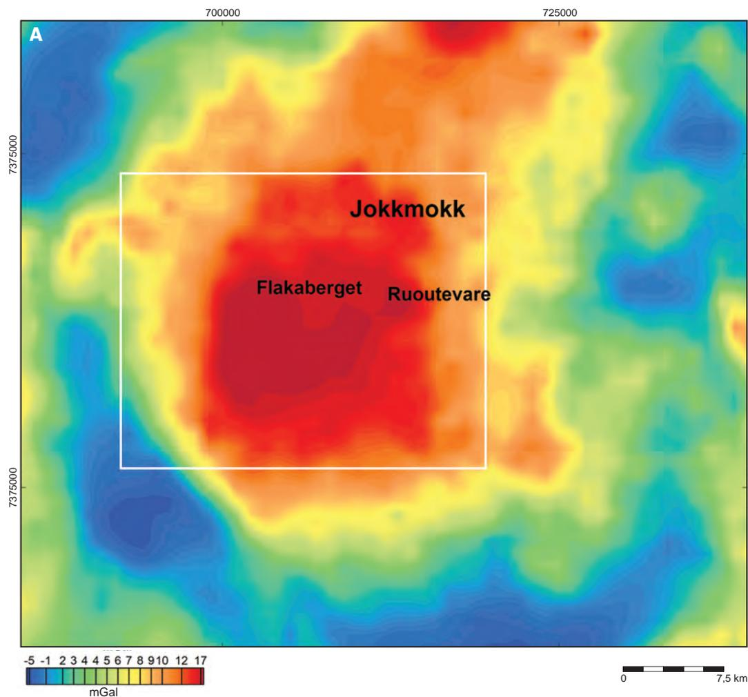
Figure 75. **A.** Bouguer anomaly map of the most prominent positive gravity anomaly in the project area. The white rectangle shows the position of the model in the horizontal plane. The location of the model area is shown in Figure 16.
