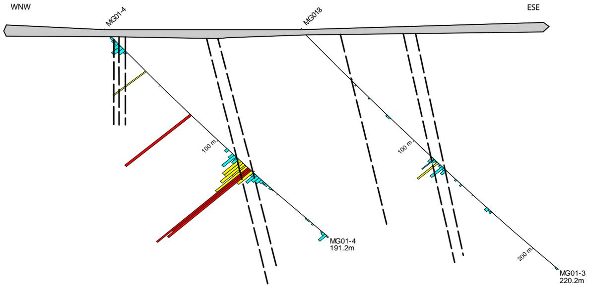
Figure 180. Zn-Pb-Ag anomalies from cored boreholes at Särkevare, peak levels in the image are at 1.65% Zn, 0.64% Pb, and 5,5 ppm Ag. Image from BHP-Intrepid.
