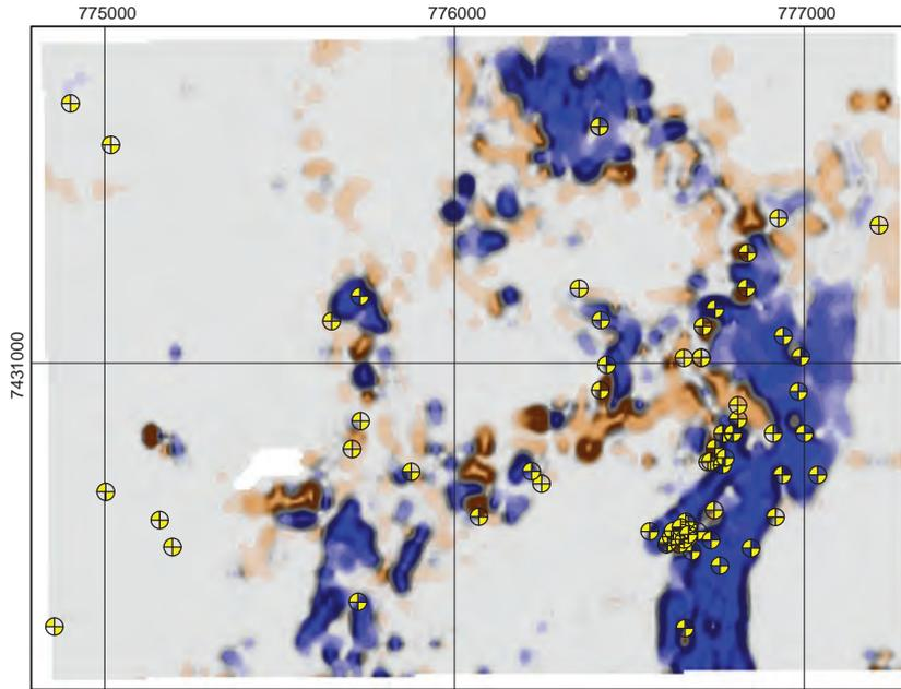
Figure 179. Electromagnetic (slingram) anomaly map at Puolalaki, imaginary component based on ground measurements. Shades of blue indicate high conductivity. The yellow symbols show the location of the drill holes.
