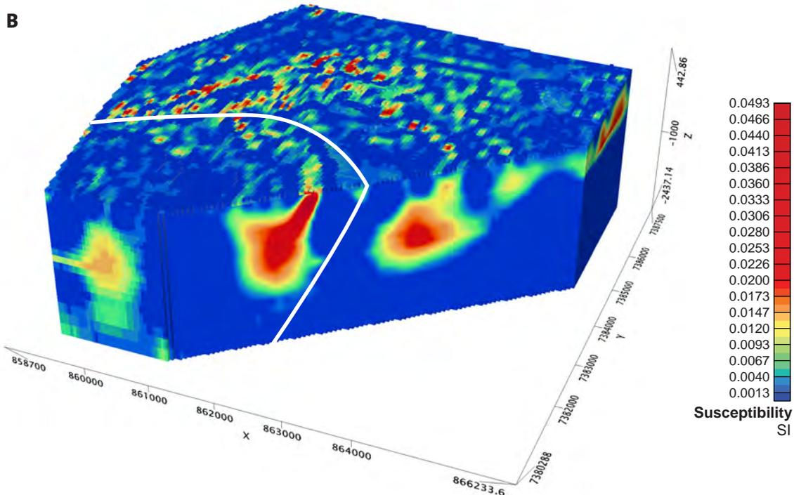
Figure 116. **B.** View from southeast of 3D susceptibility model from airborne measurements of the magnetic anomaly field. The cell size was set at 50 metres in the horizontal directions and 25 metres in the vertical direction. The white line shows an interpretation of the axial trace of the  $F_2$  fold. The location of the model is shown with the black polygon in Figure 116a and in Figure 16.
