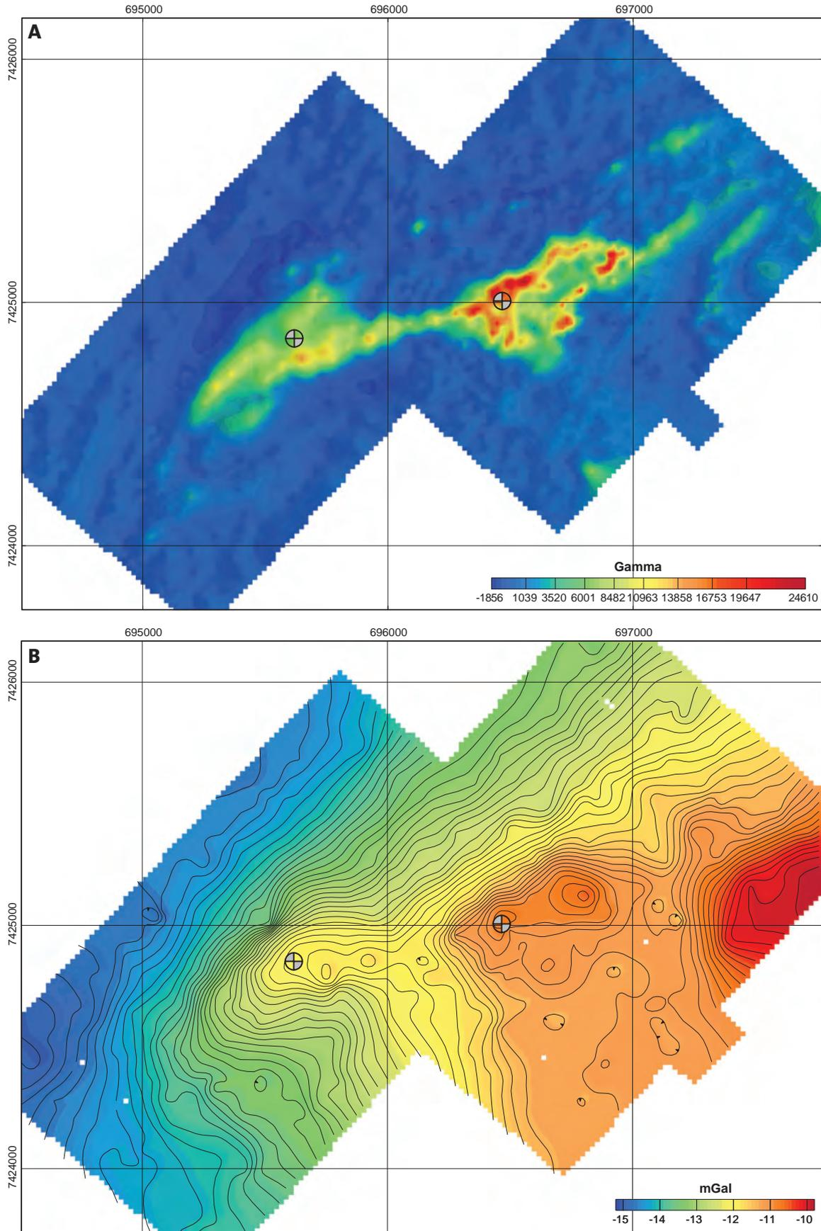
Figure 167. Geophysical anomaly maps of the Åkosjegge area based on ground measurements. The circles show the location of the drill holes. **A.** Magnetic anomaly map, vertical component. **B.** Gravity anomaly map.
