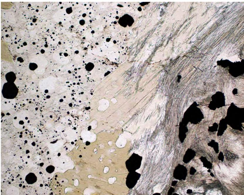
Figure 140. Paragneiss from Luspevaratj showing fibrous sillimanite to the right, altered cordierite with rounded opaque inclusions to the left, and biotite in the centre. Polarised light with parallel nicol; the long side of the image is approximately 1.4 mm (7395441/668533). Photomicrograph: Fredrik Hellström.
