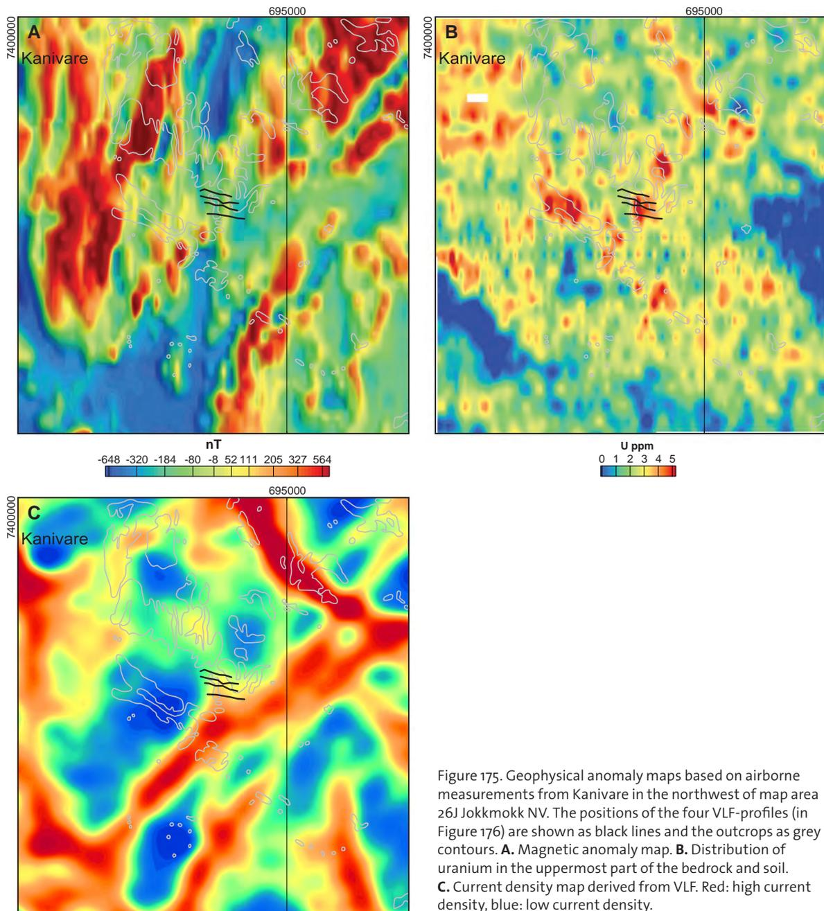
Figure 175. Geophysical anomaly maps based on airborne measurements from Kanivare in the northwest of map area 26J Jokkmokk NV. The positions of the four VLF-profiles (in Figure 176) are shown as black lines and the outcrops as grey contours. **A.** Magnetic anomaly map. **B.** Distribution of uranium in the uppermost part of the bedrock and soil. **C.** Current density map derived from VLF. Red: high current density, blue: low current density.
