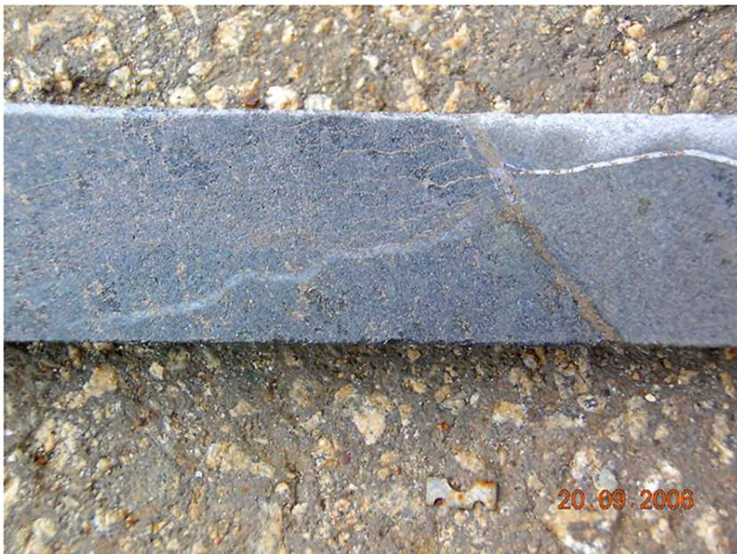
Figure 181. Altered wacke to mudstone with pyrite, sphalerite and galena in veinlets and fractures in drill core from Särkevare. Photo: BHP-Intrepid.
