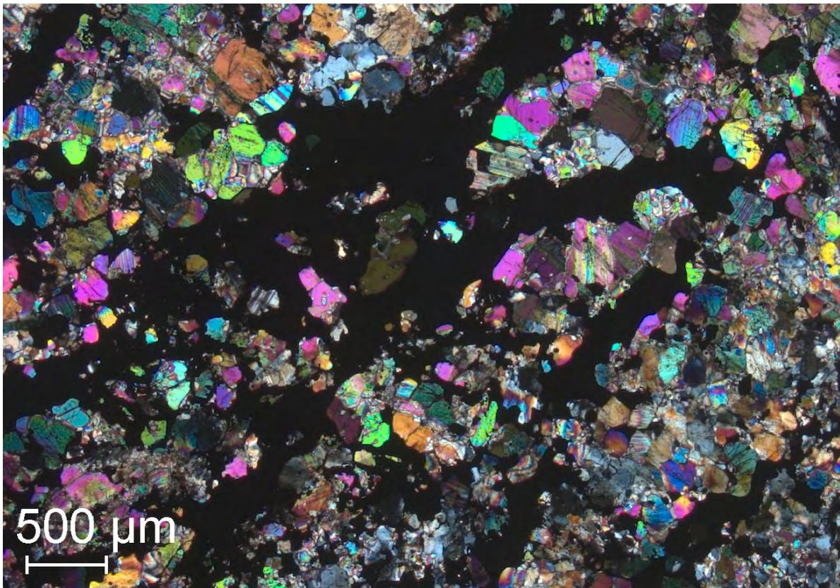
Figure 174. Clinopyroxene and pyrrhotite in a thin section from the iron-sulphide mineralisation at Kanivare, plane-polarised light, crossed nicols (7397813/694183). Photomicrograph: Dick Claeson.
