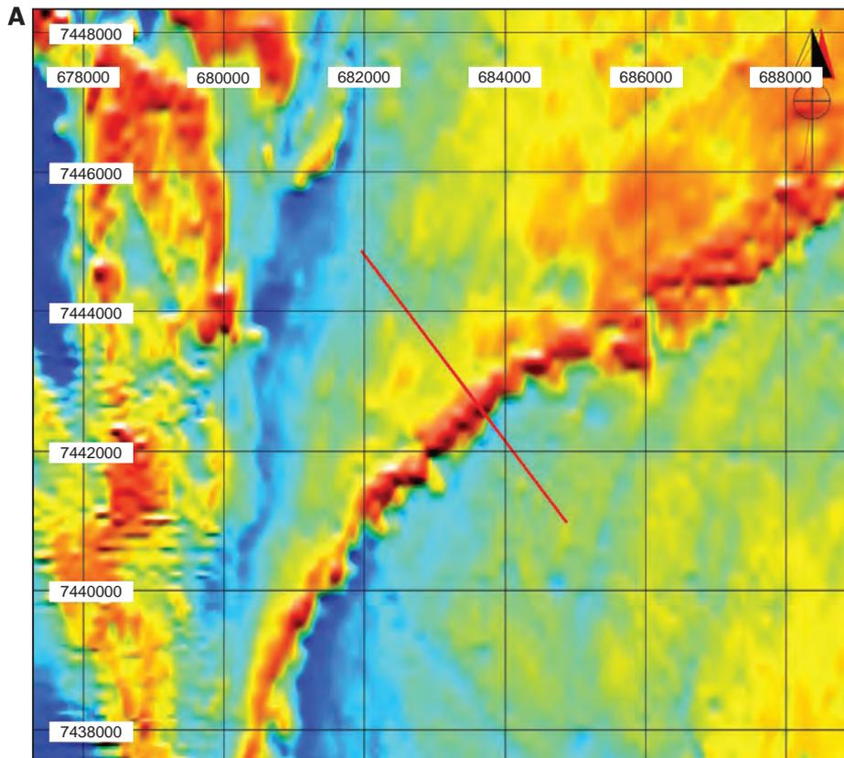
Figure 82. **A.** Magnetic anomaly map of a part of the Nabrenjarka dolerite. The profile for modelling is indicated by a red line. The location of the model area is shown in Figure 16.
