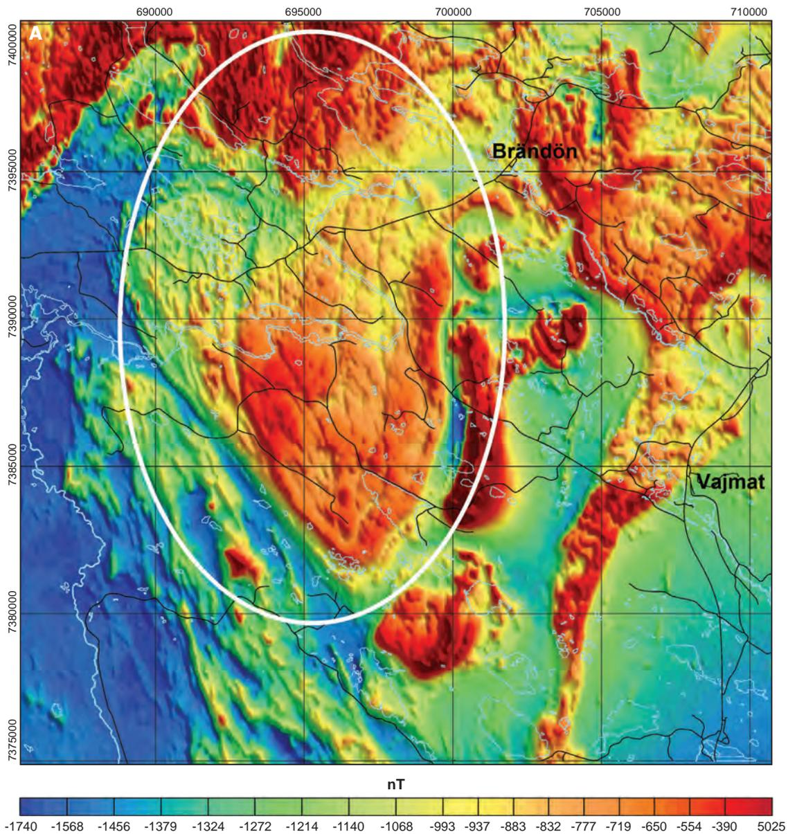
Figure 30. **A.** Magnetic anomaly map of the Noarvejávrrre area. The heart-shaped Norvijaur intrusion is marked with a white ellipsoid. The location of the model area is shown in Figure 16.
