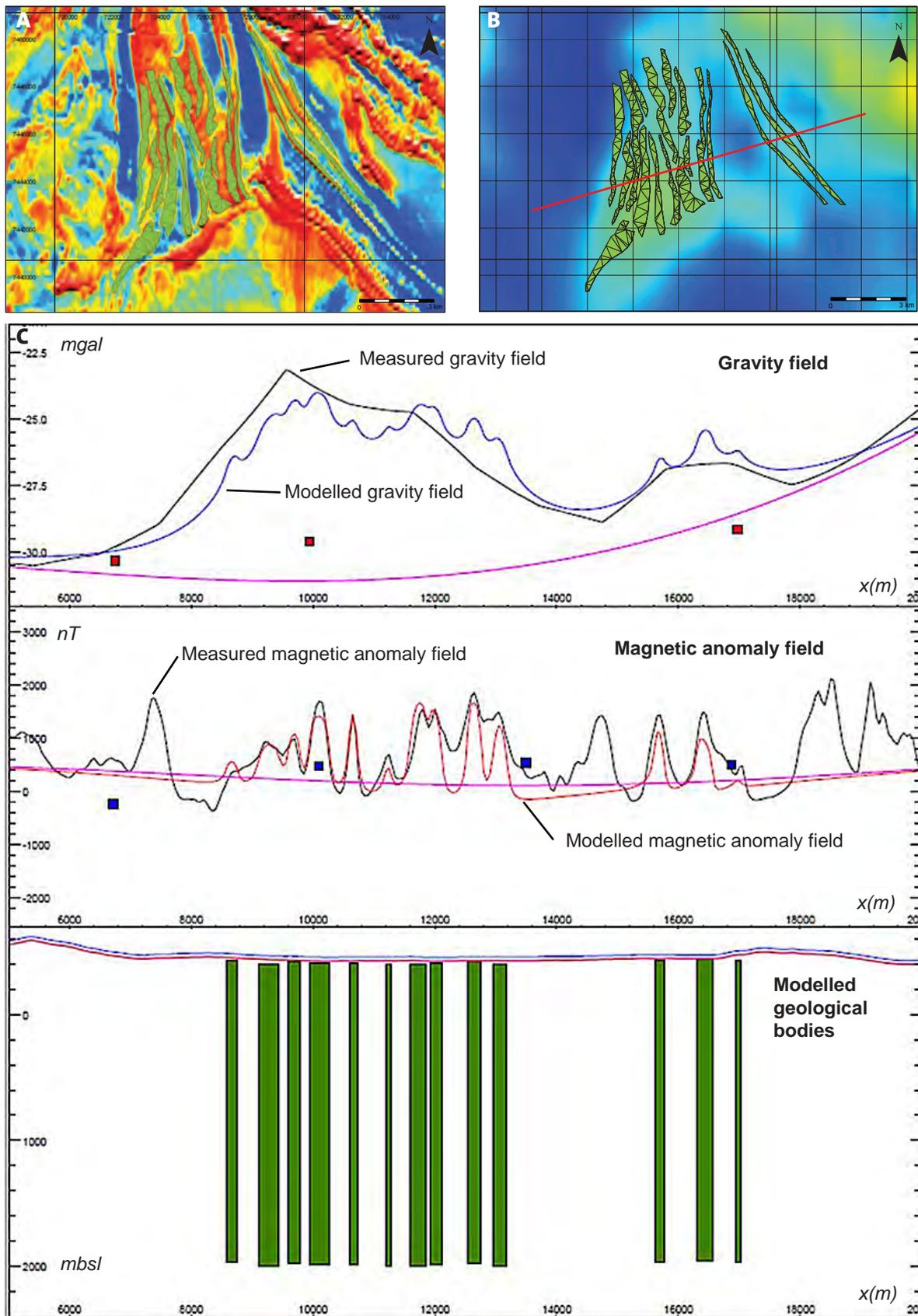
Figure 55. **A.** Filtered magnetic total field with modelled profile and source bodies. Red colours: high magnetic anomalies, blue colours: low magnetic anomalies. The location of the model area is shown in figure 16. **B.** Filtered gravity field with location of the modelled profile (red line) and the source bodies (green fields). Yellow and green colours: mass excess, bluish colours: mass deficiency. **C.** Modelling result of the gravity and magnetic field presented as a profile.
