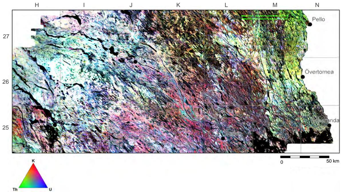
Figure 6. Radiometric map based on airborne measurements; red = potassium, blue = uranium, green = thorium.
