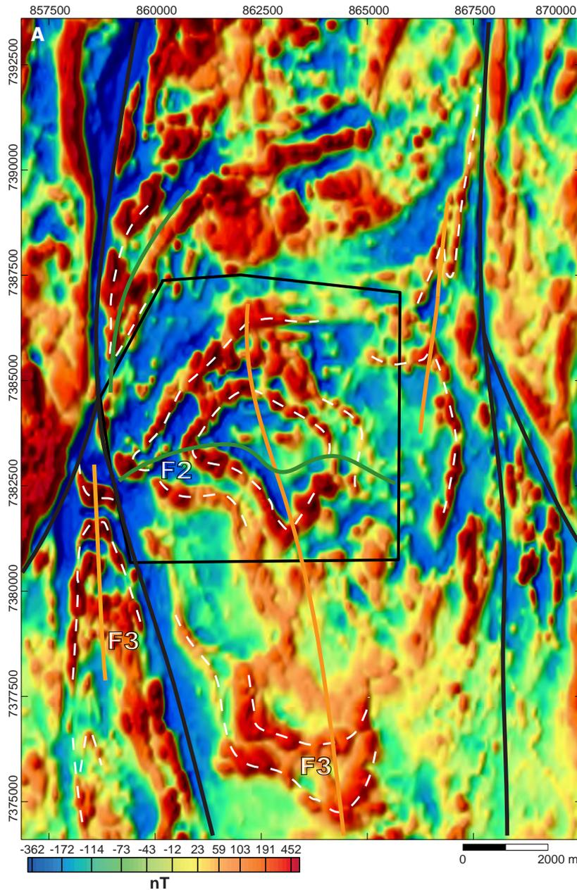
Figure 116. **A.** Fold interference pattern east-northeast of Överkalix interpreted from magnetic anomaly data. The magnetic field is filtered to enhance the shallow source anomalies. Broken white lines are magnetic connections; green and orange lines are fold axial traces of  $F_2$  and  $F_3$ , respectively, and black lines are deformation zones.
