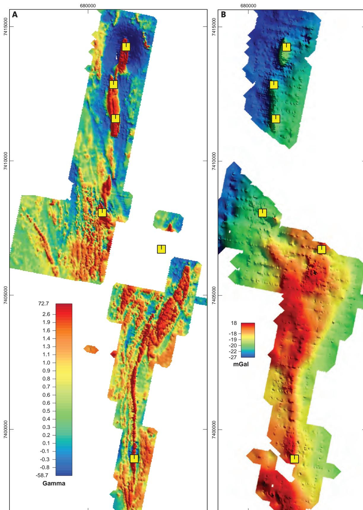
Figure 166. Geophysical anomaly maps of the Kallak area based on ground measurements. The iron oxide mineralisations (ore) are shown as yellow squares. **A.** Magnetic anomaly map, vertical component. **B.** Terrain-corrected Bouguer anomaly map.
