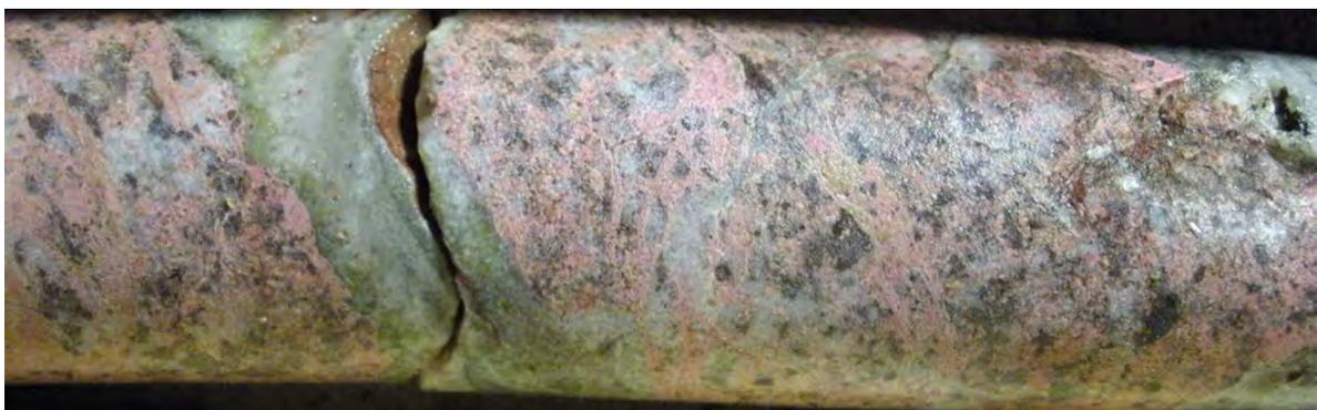
Figure 135. Zone where the rock is brecciated with traversing quartz-filled fractures and extensive red to pink pigmentation. Drill core from Svikkomaa. Photo: Dick Claeson.
