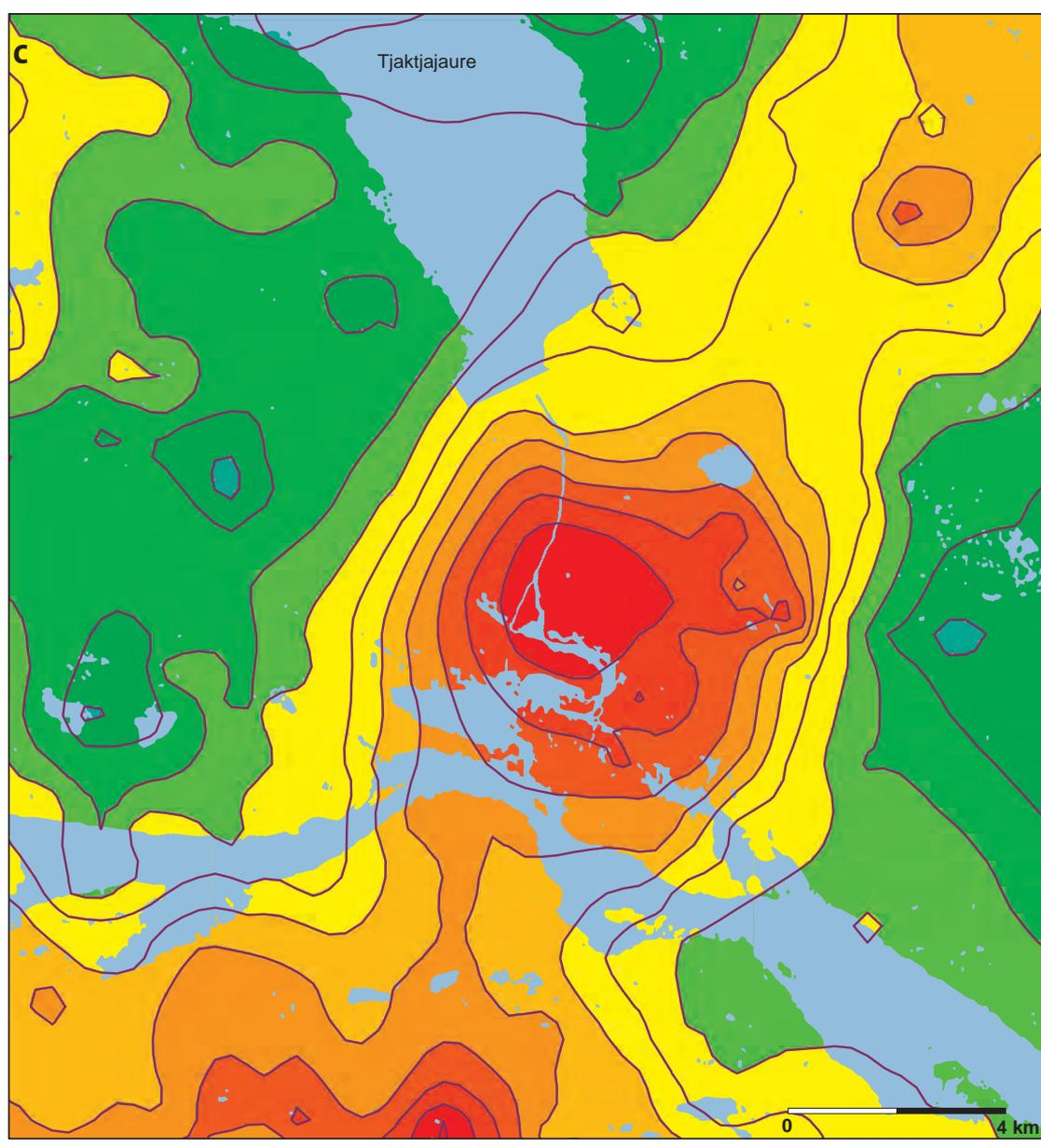
Figure 75. C. Gravity anomaly adjacent to the Tjaktjajaure dam. The figure shows a filtered gravity field of the area. Reddish colours represent gravity high and green colours gravity low.
