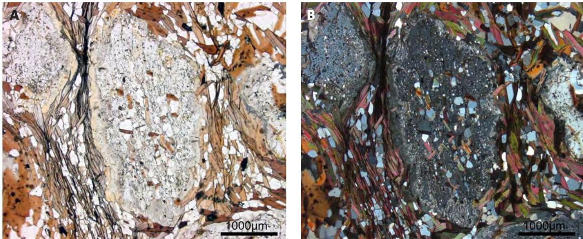
Figure 148. Alteration in fractures and at the edges of cordierite crystals with formation of yellowish pinite. **A.** Plane polarised light. **B.** Crossed nicols (7376949/731144). Photomicrograph: Dick Claeson.
