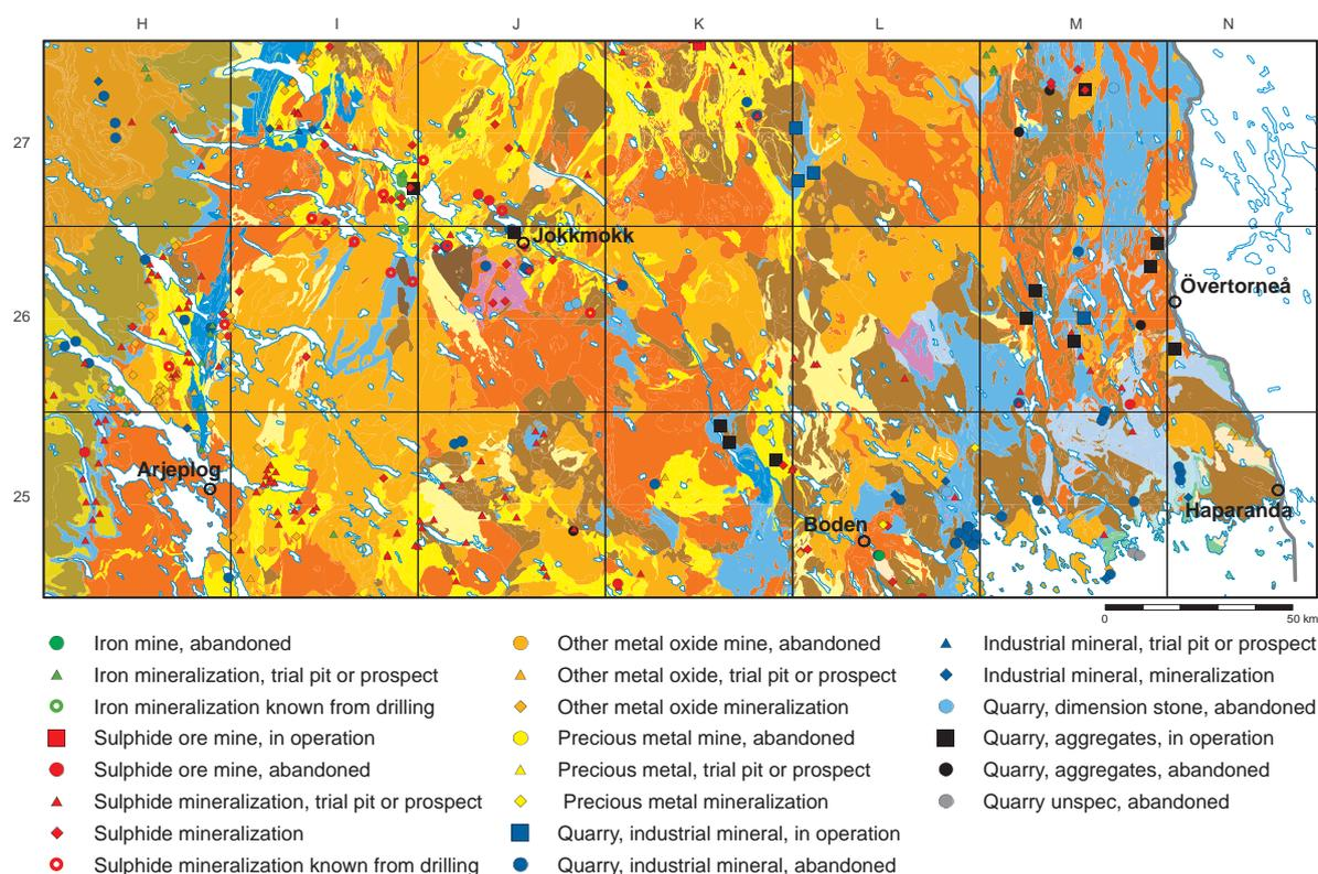
Figure 154. Distribution of the principal types of metallic and non-metallic mineral deposits in southern Norrbotten County. The deposits are presented on a simplified bedrock geological map. Geological units as in Figure 17b.
