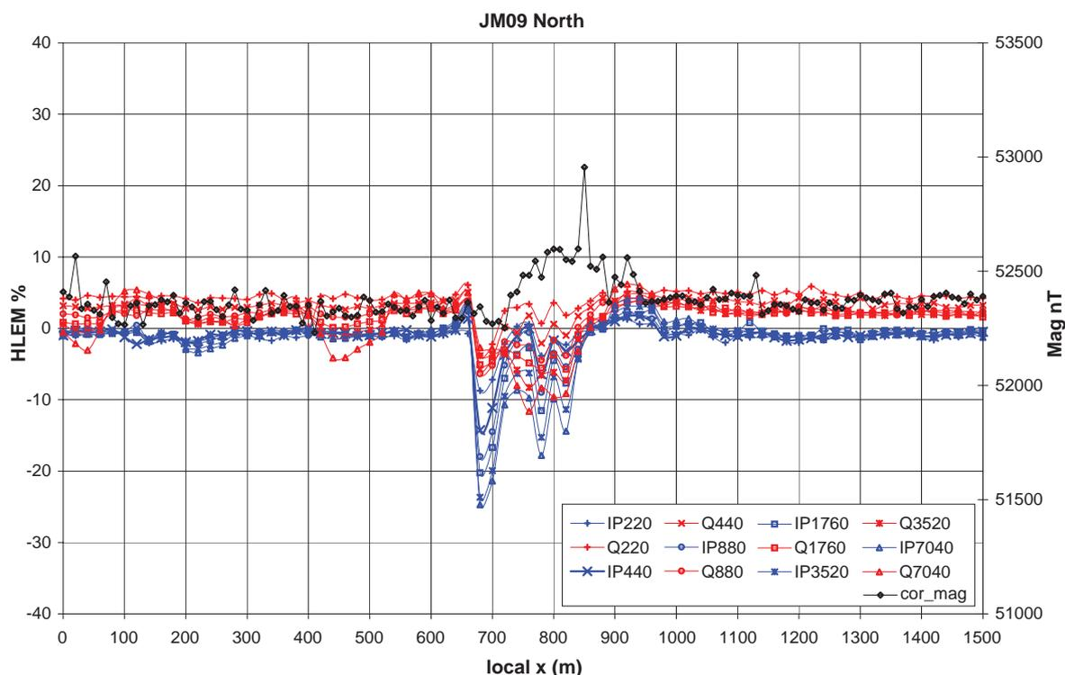
Figure 178. One of the ground electromagnetic measurements (EM) of the drilled anomaly in the Tjerkisberget area. A black line shows the magnetic field. The red and blue lines show real (IP) and imaginary (Q) component from the horizontal loop multifrequency EM measurements. The measurements were made by Suomen Malmi Oy (Lahti 2004). The magnetic and EM anomalies coincide well except for the first EM anomaly, which has a low magnetic signature.
