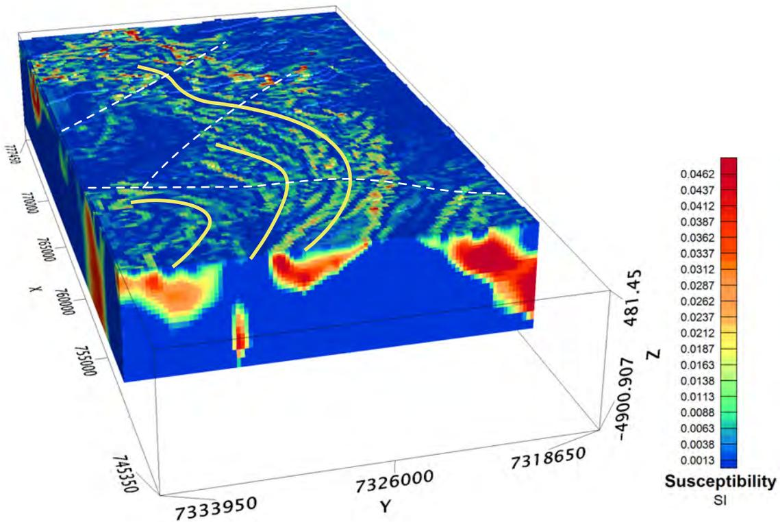
Figure 113. 3D susceptibility model from airborne measurements of the magnetic anomaly field southwest of Harads. The cell size was set to 150 metres in the horizontal directions and 75 metres in the vertical direction. The area of the model is 32 x 15 kilometres. Yellow lines are axial surface traces of F<sub>2</sub> folds and broken white lines are deformation zones. View looking down to the east-southeast. The location of the model is shown in Figure 16.
