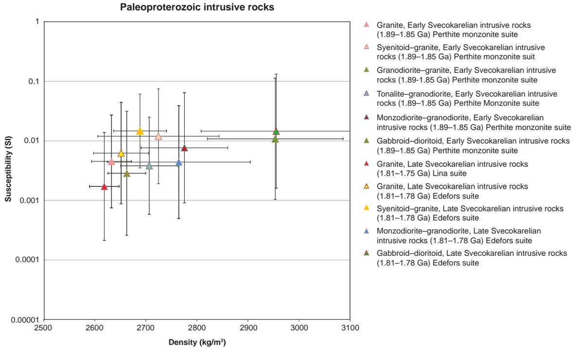
Figure 104. Magnetic susceptibility v. density for Palaeoproterozoic intrusive rocks.
