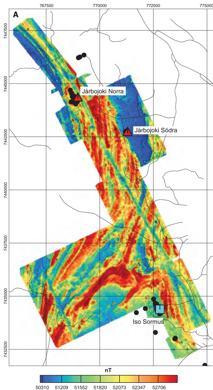
Figure 156. Ground geophysical measurements of the Järbojoki–Iso Sormus area. The measurements were made with a line distance of 80 m and point distance of 20 m. **A.** Magnetic total field. Round symbols show the location of the drill holes. Red triangles show the locations of the Järbojoki Norra and Järbojoki Södra sulphide mineralisations; the blue square shows the location of the olivine-serpentine deposit at Iso Sormus.
