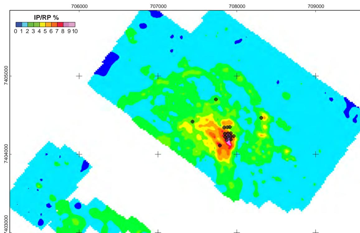
Figure 158. Induced polarisation at Vaikijaur. Black symbols (circles) show the location of the drill holes on IP anomalies.
