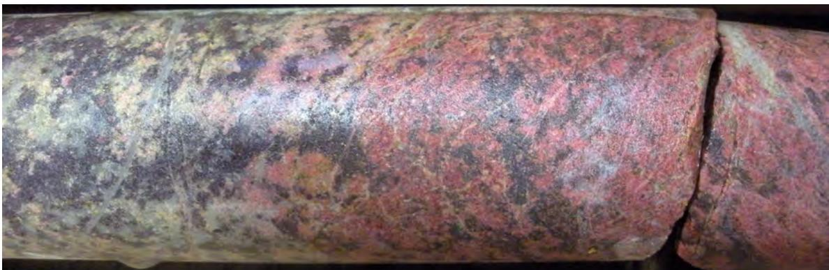
Figure 134. Red pigmented, extensively altered quartz monzodiorite, brecciated and with quartz-filled fractures. Drill core from Svikkomaa. Photo: Dick Claeson.
