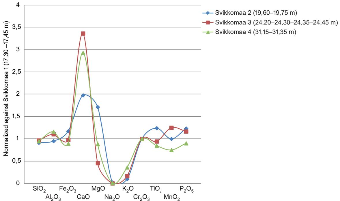
Figure 137. Plot of severely altered rock samples from the drill core at Svikkomaa, normalised against a rock sample of well-preserved monzodiorite from the same drill core.
