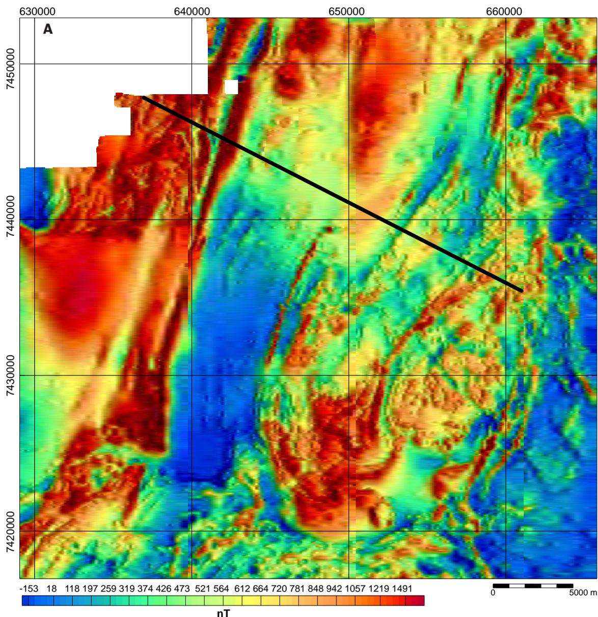
Figure 118. A. Magnetic anomaly map of the Tjåmotis area. The black line shows the position of the modelled profile in Figure 118b. The profile length is approximately 28 kilometres.
