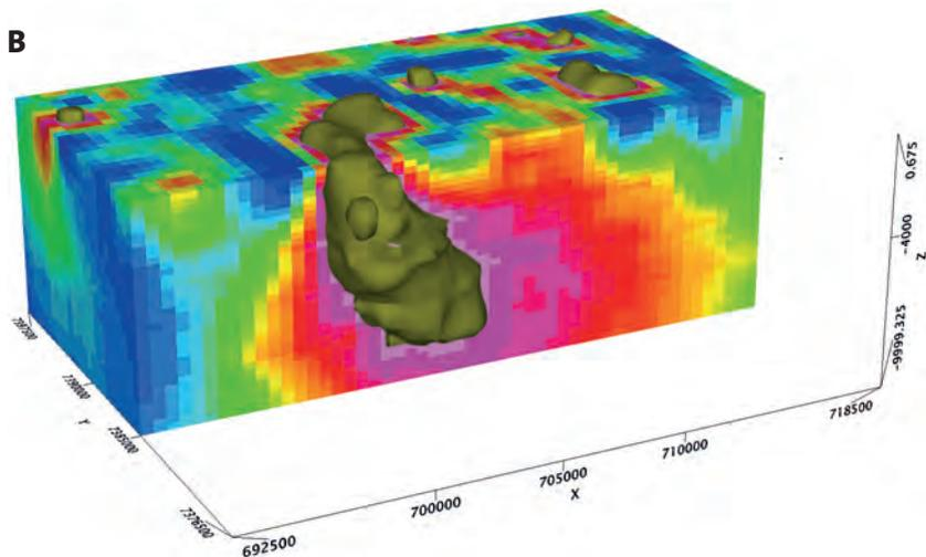
Figure 75. B. The 3D density model of the study area. The isosurface corresponds to density values of 2900 kg/m<sup>3</sup> and is assumed to delineate gabbroids. The isosurface is shown in brown.
