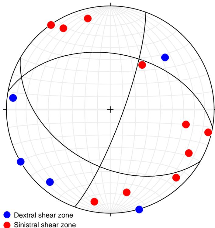
Figure 127. Stereogram (Schmidt projection, lower hemisphere) of poles to boundaries of ductile strike-slip shear zones in the area east of the KADZ and south of Jokkmokk. Dextral (blue) and sinistral (red) shear zones separate into quadrants indicating approximately west-northwest extension or moderately south-plunging shortening (190/45).
