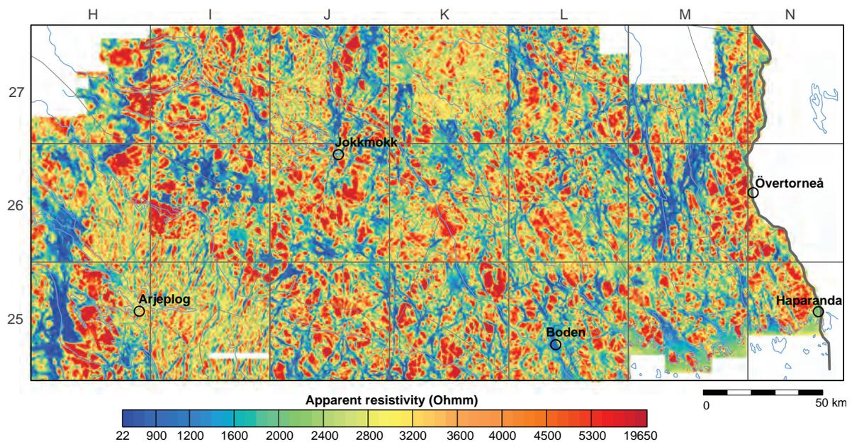
Figure 7. Map of resistivity based on airborne VLF measurements.
