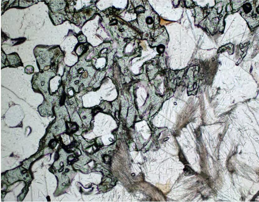
Figure 141. Green spinel in paragneiss from Luspevaratj with quartz. Needles of fibrous sillimanite seen to the right. Polarised light with parallel nicol; the long side of the image is approximately 1.4 mm (7395441/668533). Photomicrograph: Fredrik Hellström.
