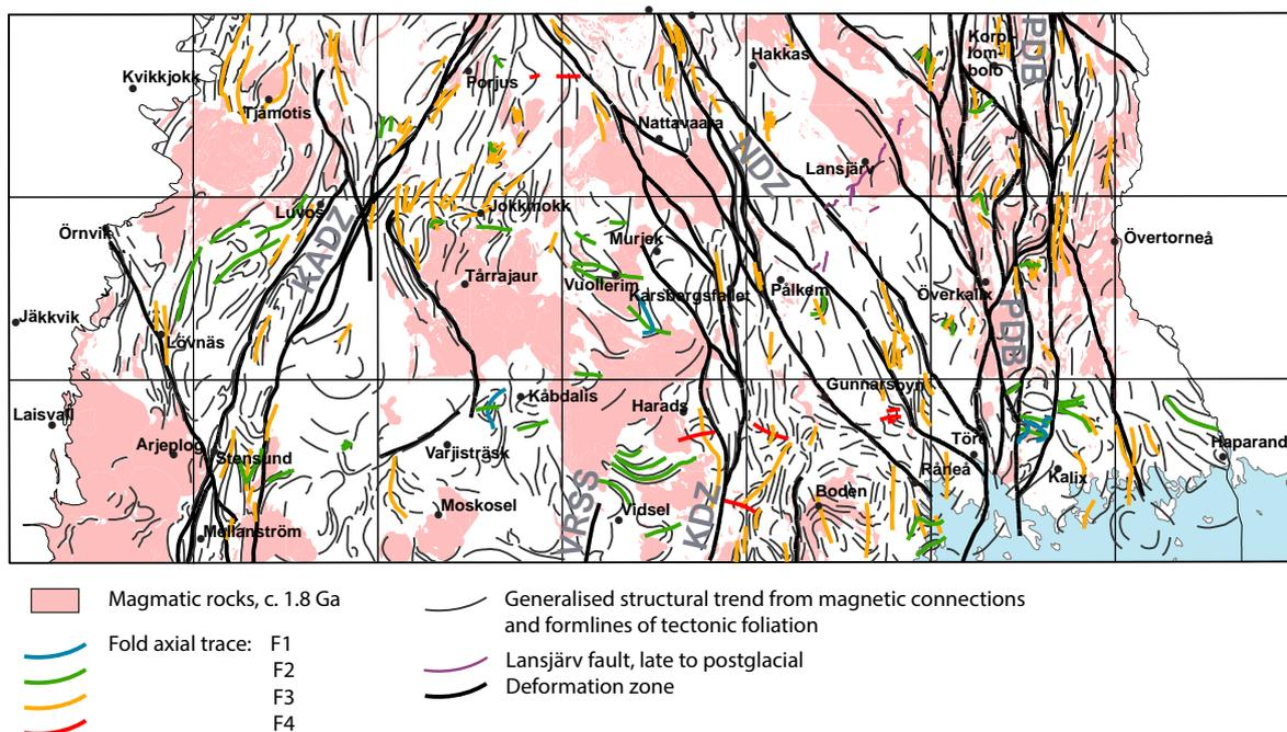
Figure 110. Generalised structural trends displayed by form lines of tectonic foliation as well as magnetic connections that are interpreted to represent tectonic foliation and the main ductile shear zones. Fold axial traces are indicated with thick lines whose colour denotes their relative age. KADZ = Karesuando–Arjeplog deformation zone, NDZ = Nautanen deformation zone, PDB = Pajala deformation belt, VRSS = Vidsel–Röjnoret shear system, KDZ = Karsbergfallet deformation zone.
