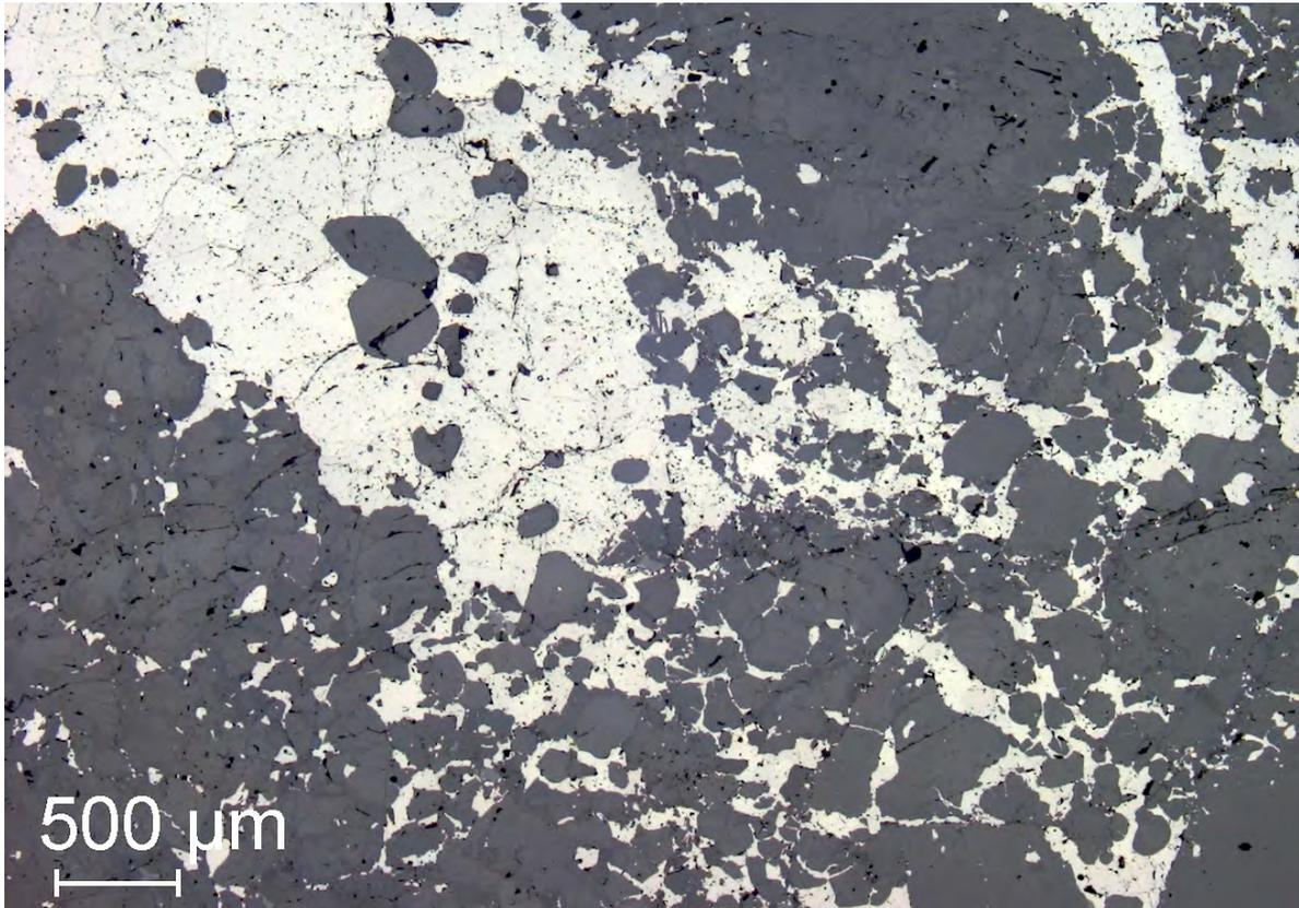
Figure 173. Pyrrhotite (bright) and silicate minerals (grey) in a thin section from the iron-sulphide mineralisation at Kanivare, reflected light (7397813/694183). Photomicrograph: Dick Claeson.
