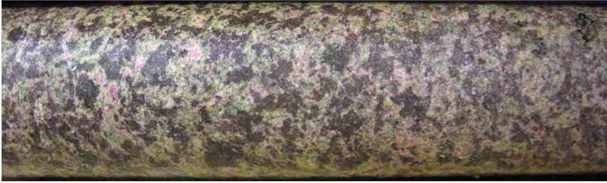
Figure 136. Green and red pigmented, significantly altered quartz monzodiorite. Drill core from Svikkomaa. Photo: Dick Claeson.
