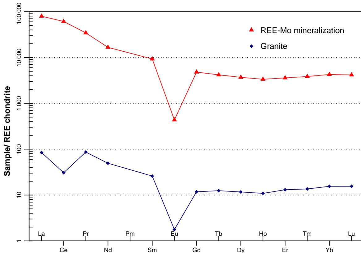
Figure 183. REE diagram with data from lithochemical analyses of granite and the REE-Mo mineralisation at Tåresåive. Normalising values for chondrite from Boynton (1984).
