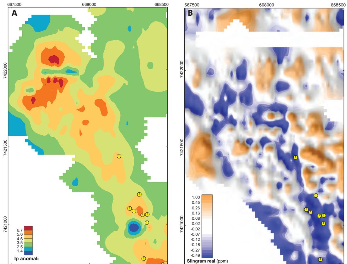
Figure 172. Geophysical anomaly maps based on ground geophysical measurements at Tjäula. Locations of drill holes are shown with yellow symbols. **A.** Induced polarisation (IP). **B.** Slingram, real component.
