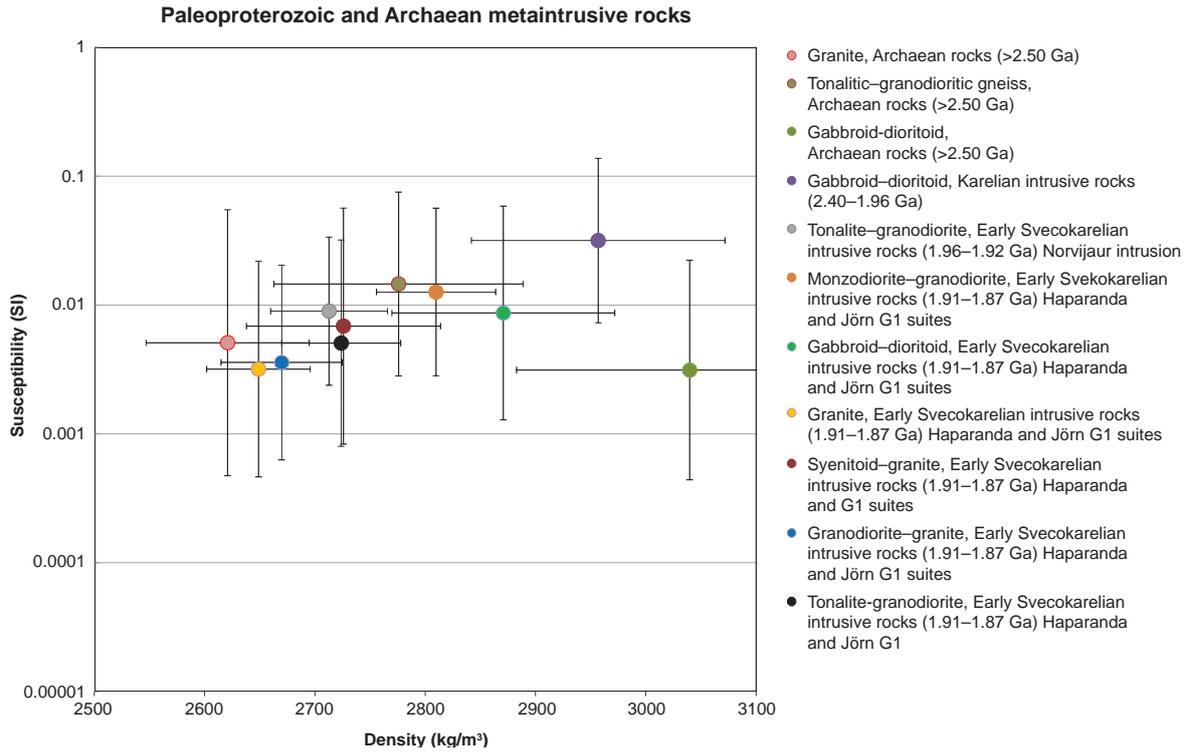
Figure 102. Magnetic susceptibility v. density for Palaeoproterozoic and Archaean metaintrusive rocks.
