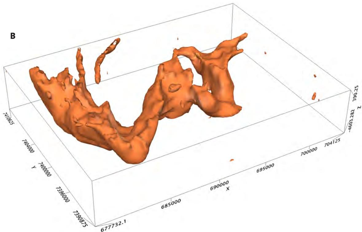
Figure 117. **A.** Major  $F_3$  folds shown in the total magnetic field of the area west of Jokkmokk. **B.** Susceptibility model of gently north-plunging  $F_3$  folds, presented as a susceptibility isosurface of 0.05 SI. View looking down towards the northeast. The cell size was set at 250 metres in the horizontal directions and 125 metres in the vertical direction. The location of the model is shown in Figure 16.
