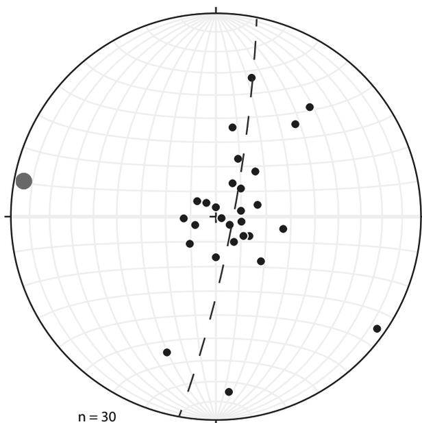
Figure 114. Equal area stereographic plots (lower hemisphere) of poles to bedding in the metavolcanic and metasedimentary rocks in the area southwest of Harads. The broken line is the best fit great circle, and the grey dot is the  $\pi$ -axis. The latter and the fold axis in the 3D model (Figure 113) have similar orientations.
