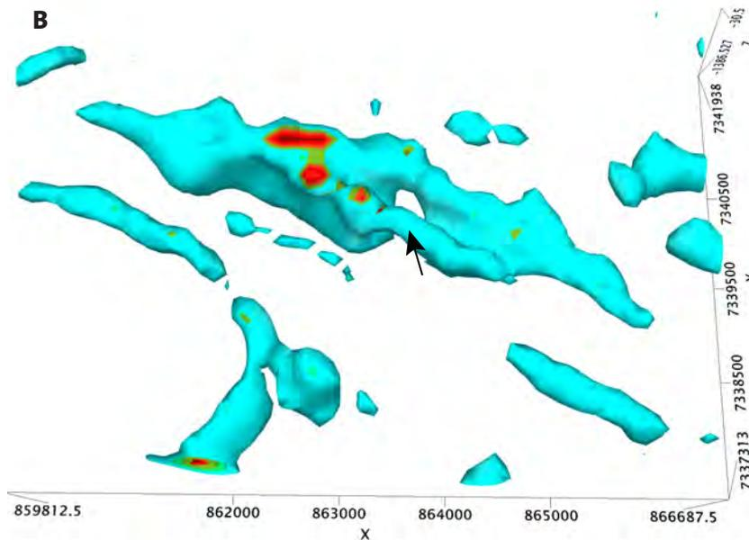
Figure 115. **B.** Susceptibility model of the gently plunging, isoclinal  $F_1$  synform (black arrow) in the central part of A, presented as a susceptibility isosurface of 0.03 SI. View looking down towards the northwest. The cell size was set at 125 metres in the horizontal directions and 75 metres in the vertical direction. The location of the model is shown with the black square in Figure 115a, and in Figure 16.
