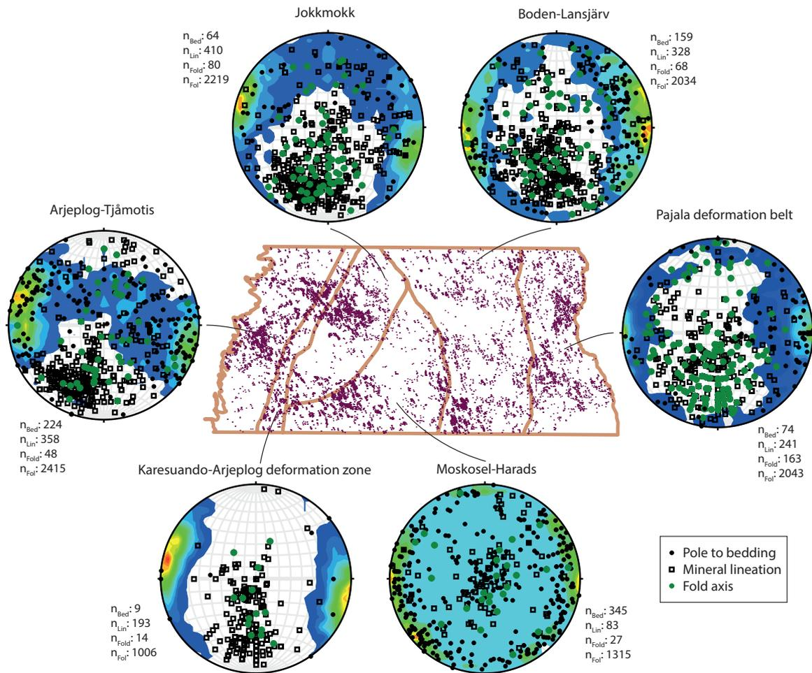
Figure 111. Equal area stereographic plots (lower hemisphere) of field measurements of planar and linear structures from the structural domains. The contours represent poles to foliation. The structural domains and locations of the structural measurements are shown on the map. The number of measurements are indicated by the following abbreviations: Bed = bedding, Lin = mineral lineation, Fold = fold axis, Fol = foliation.
