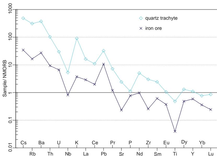
Figure 165. Multi-element diagram with data from lithochemical analyses of the quartz trachyte host rock and the iron ore at Kallak. Normalising values for N-MORB from Sun & McDonough (1989).
