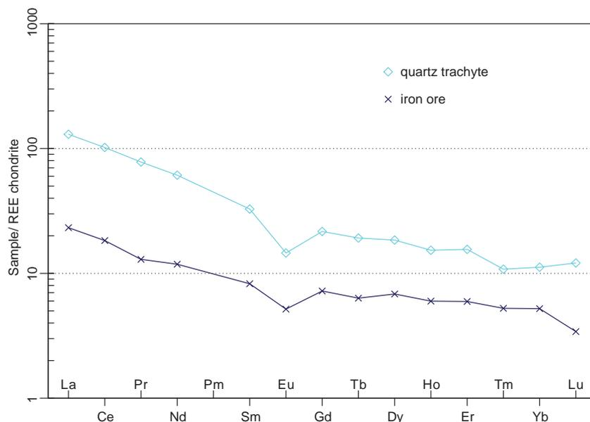
Figure 164. REE diagram with data from lithochemical analyses of the quartz trachyte host rock and the iron ore at Kallak. Normalising values for chondrite from Boynton (1984).
