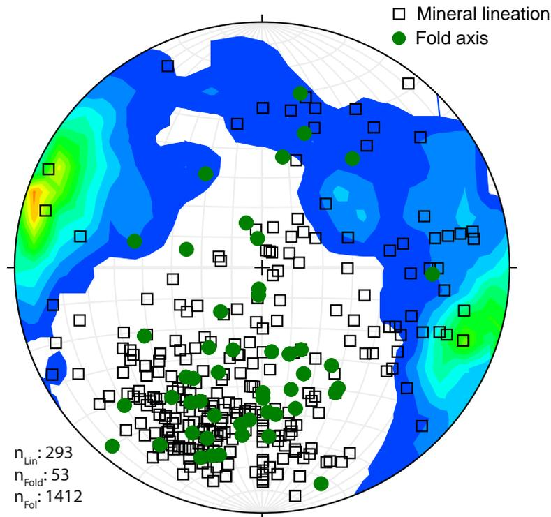
Figure 123. Orientations of structural data from the Jokkmokk area. Equal area stereographic plots (lower hemisphere) of lineations and fold axes. Contours of poles to foliation are shown in blue to red colours. The number of measurements are indicated by the following abbreviations: Lin = mineral lineation, Fold = fold axis, Fol = foliation.
