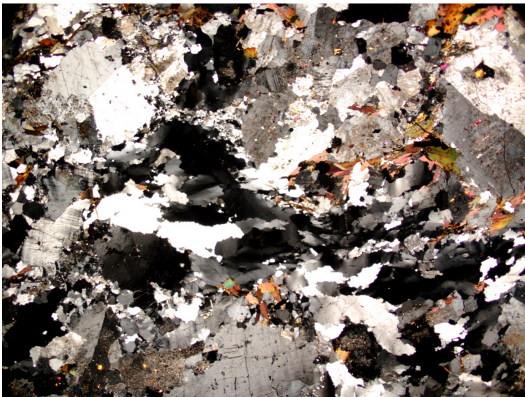
Figur 4 C. Photomicrograph of the dated sample. Domains of elongate aggregates of recrystallised quartz and minor feldspar define a tectonic foliation between less deformed domains with megacrysts of K-feldspar and plagioclase. Crossed nicols. The long dimension of the photograph is c. 12 mm.
