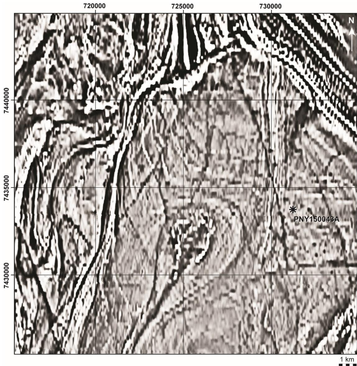
Figure 2. Map of the total magnetic field (vertical derivative). High magnetic anomalies are shown in light grey and low in dark grey.
