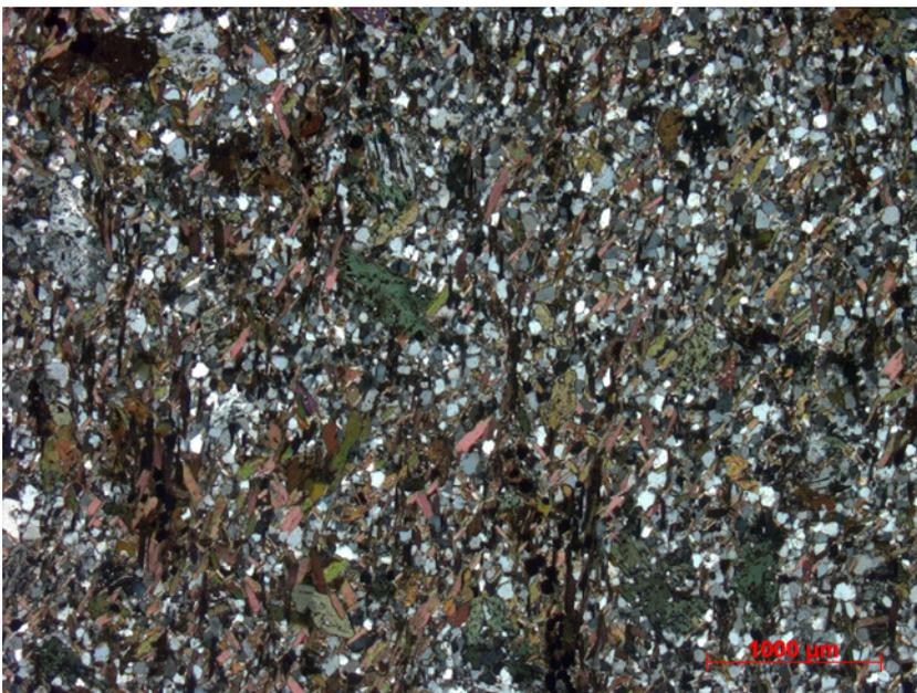
**Figure 18.** Andesite from the road cut at Solfallet, about 4 km northwest of Norberg (6661770/548370). Crossed nicols. Microphotograph: Benno Kathol.
