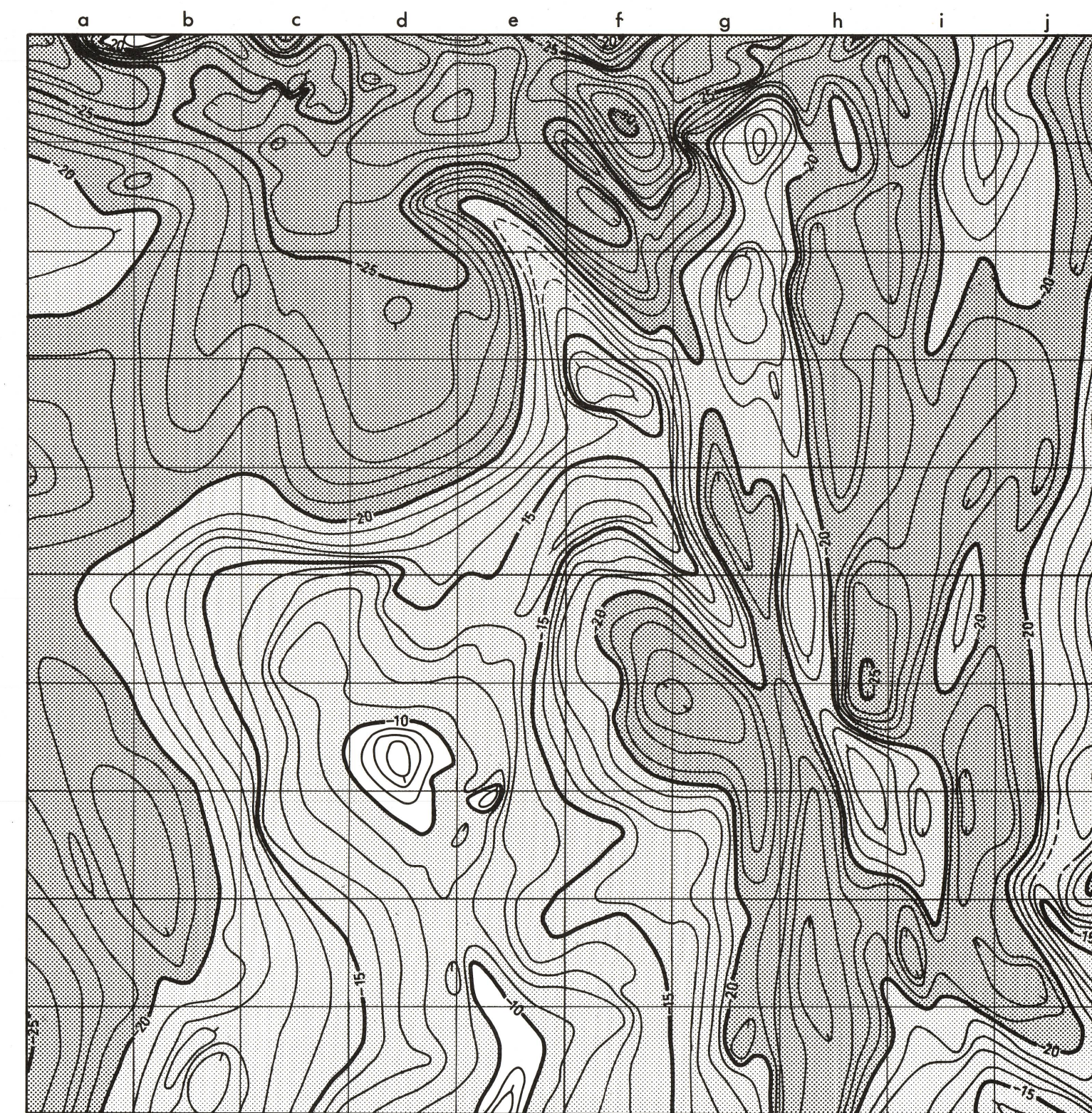
C. GRAVITY TYNGDKRAFT SCALE 1:250.000 0 5 10 km BOUGUER ANOMALY BOUGUER ANOMALI contour interval: 1 mgal 5 mgal ekvidistans -10 mgal -20 -30 minima minimum maxima maximum REFERENCE SYSTEM REFERENSSYSTEM ECS 62 international formula 1930 internationell formel 1930 Bouguer density 2.67 Bouguer täthet 2.67 terrain correction applied terrängkorrigerad
