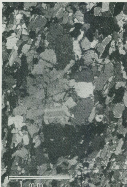
Fig. 28. Amphibolite: a magmatic plagioclase crystal replaced by an aggregate of roughly equant, metamorphic plagioclase crystals.
