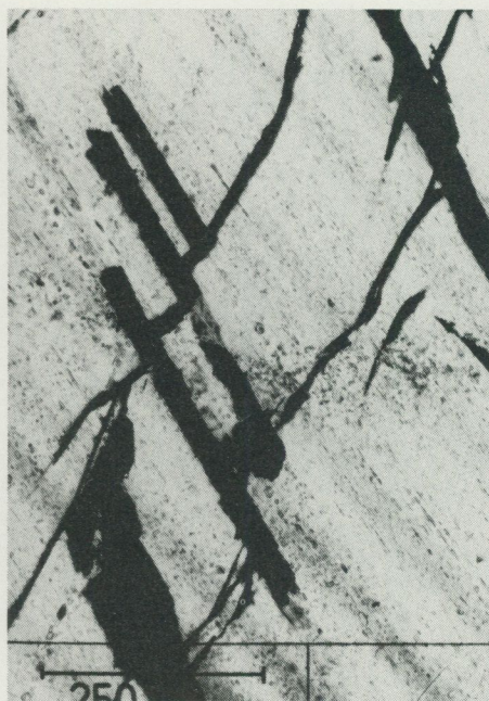
Fig. 20. Plagioclase showing cracks filled with opaque material (crossed polars); gabbroic Hyperite.
