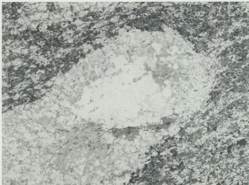
Fig. 27. Amygdaloidal metabasite generation I. + nic., 12\times . 250 m N of Skälö. Map-sheet Vimmerby NO (7j).
