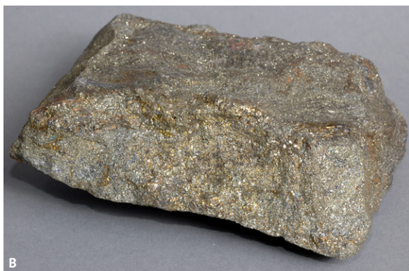
Fig. 113. Two types of base metal sulphide deposits in the Bergslagen region. A. Layered sphalerite-dominated SAS-type ore (Allen et al. 1996) from the Zinkgruvan deposit. The photograph is 12 cm wide in a horizontal direction. B. Semi-massive, chalcopyrite-pyrite SVALS-type ore (Allen et al. 1996) from the Falun deposit. The specimen is 13 cm wide in a horizontal direction. Photographs Torbjörn Bergman (SGU).
