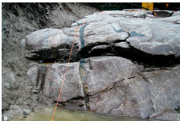
Fig. 162. Subhorizontal and gently dipping fractures close to the ground surface at Forsmark in the north-eastern part of the Bergslagen region. A. Subhorizontal fracture filled with glacial sediment (Quaternary) inferred to be a sheet joint formed in connection with release of stress close to the ground surface. Excavation at the Forsmark nuclear power plant (after Carlsson 1979). B. Gently dipping fracture with wide aperture at drill site 5, Forsmark. The impressive aperture along this fracture is also inferred to have formed in connection with the release of stress close to the ground surface. Several fractures with this orientation at drill site 5 are filled with glacial sediment (Quaternary).
