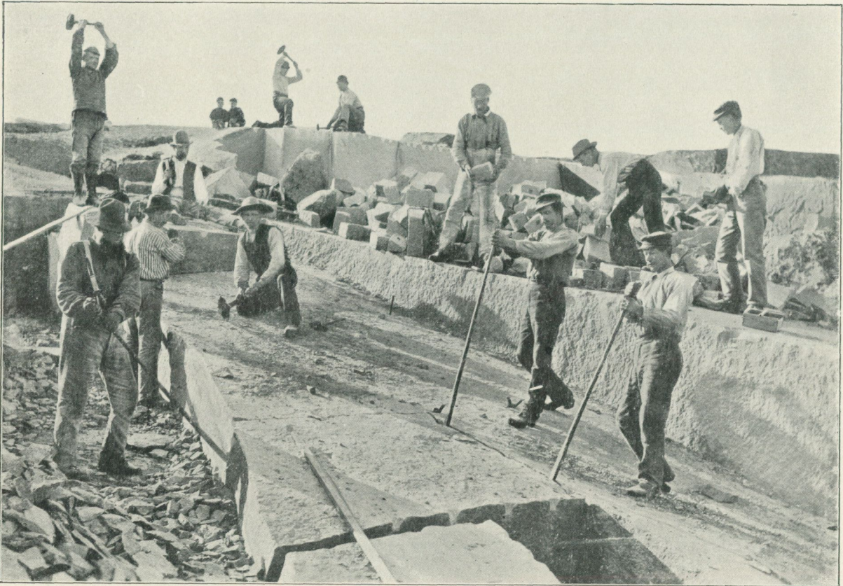
Bohuslän granite-quarry on Malmsön off Lysekil, illustrating the marked joints of the granite.
