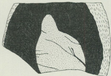
Fig. 2. Copper ore in a »sköl», Mårtanberg. \frac{3}{4} nat. size. Black is bornite, dotted chalcopyrite, short lines indicate »sköl» matter (amphibole and chlorite).
