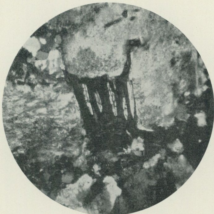
Fig. 11. Origin of microcline in altered biotite. Quartz-syenite from Aspetorp farm. Micro-photo., \times 35 . Nicols +.
