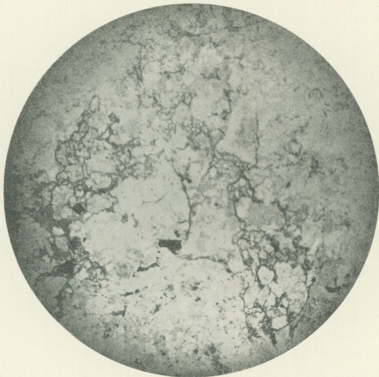
Fig. 2. Silverknut granophyre, ord. light, magn. 16 times, showing the breccia like distribution of the micas.
