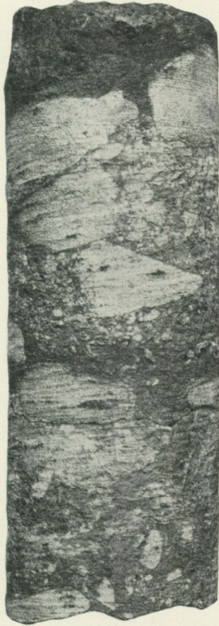
Fig. 6. Portion of [the core of the conglomerate covering the Lower Cambrian sandstone. The fine-grained, somewhat pyritic, dark-grey sandstone-matrix is larded with pebbles and more or less angular pieces of light-grey quartzite. Level: 46.15—46.40 m. — Half nat. size.
