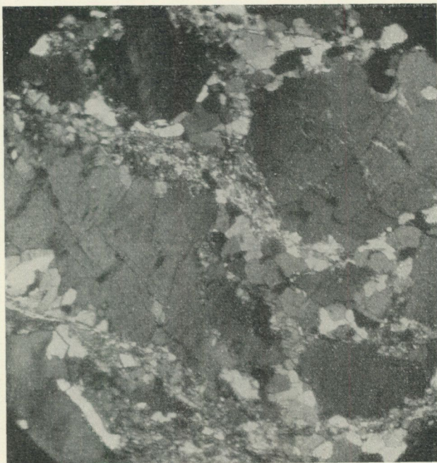
Fig. 15. Injection-granite showing partial crushing of the grains (at the rims of the large grains).
