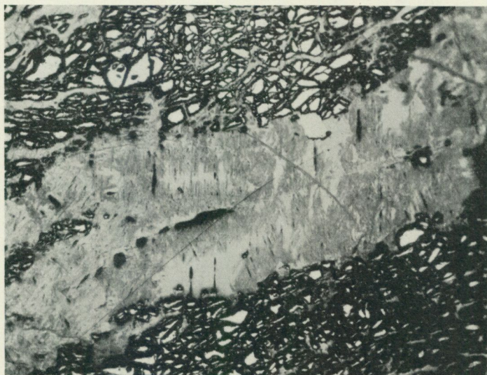
Fig. 16. Covellite (dark-gray needles) replacing chalcocite (light gray) from fissure. Chalcocite cuts and replaces pyrite (white with relief). Pol. sec., ord. light, 130 \times .
