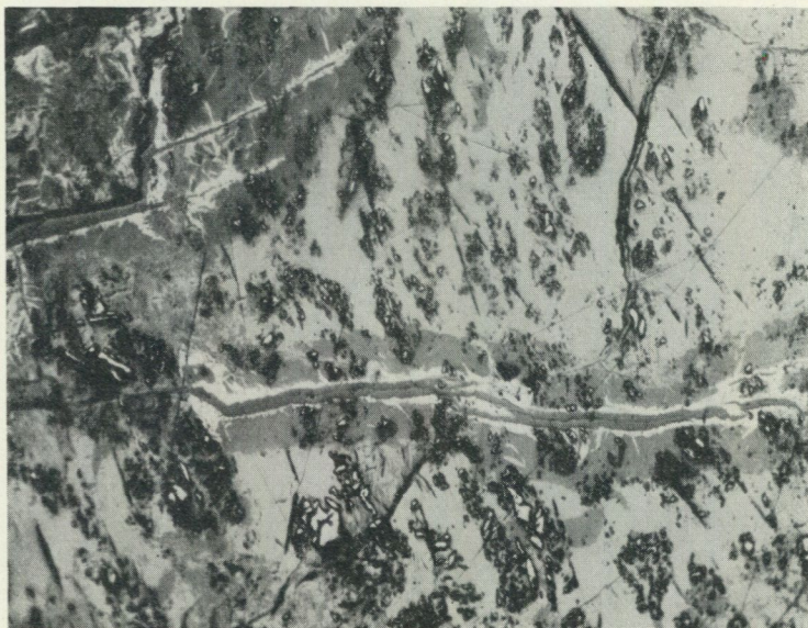
Fig. 18. "White" chalcocite with remnants of pyrite (grains with relief). In lower half and upper left veinlets of bornite (dark gray), chalcopyrite (white), and limonite (in centre of veins). Pol. sec., ord. light, 130 \times .
