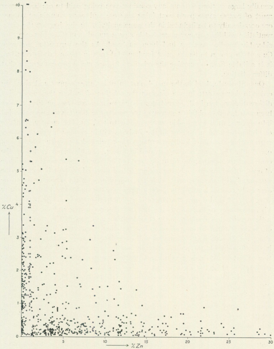
Fig. 1. Relations between Cu and Zn percentages in the Rävliiden ores. Crosses denote a number of copper-ore analyses in which Zn has not been determined, but where the Zn percentages are undoubtedly < 1\% .
