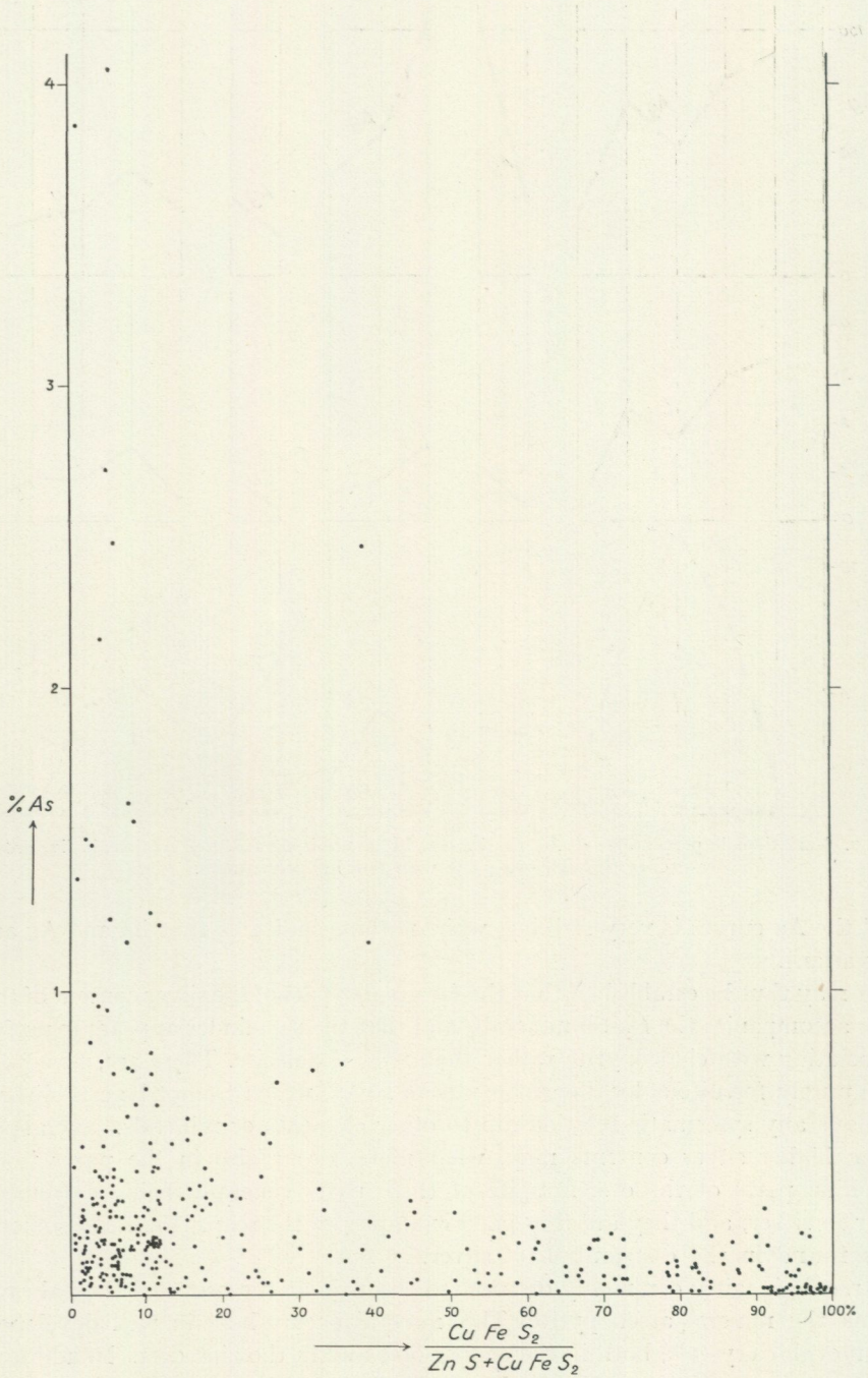
Fig. 8. Diagram showing the relations of the As percentages to the copper-zinc differentiation.
