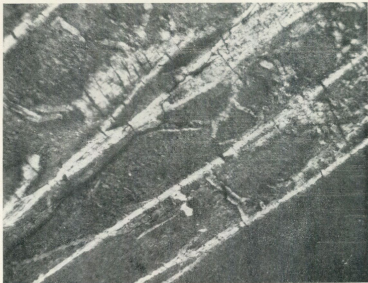
Fig. 4. Veinlets of carbon mineral in massive, fine-grained carbon with almost submicroscopic remnants of U-mineral. N crossed, 45 x. 330 m level, east.
