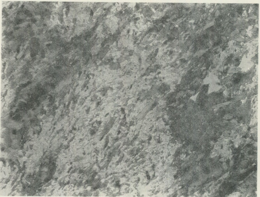
Fig. 7. Border of greenstone dyke. It is mainly remnants of liparite between biotite grains. Dark spots are halos round orthite grains. Cross-cut 20, 50 m level. 51 X, ordinary light.
