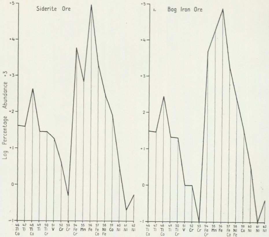
Fig. 26. Diagram of the percentage abundance of the ferride isotopes with mass-numbers 46—62 in siderite ores and in the bog iron ores of Finland.
