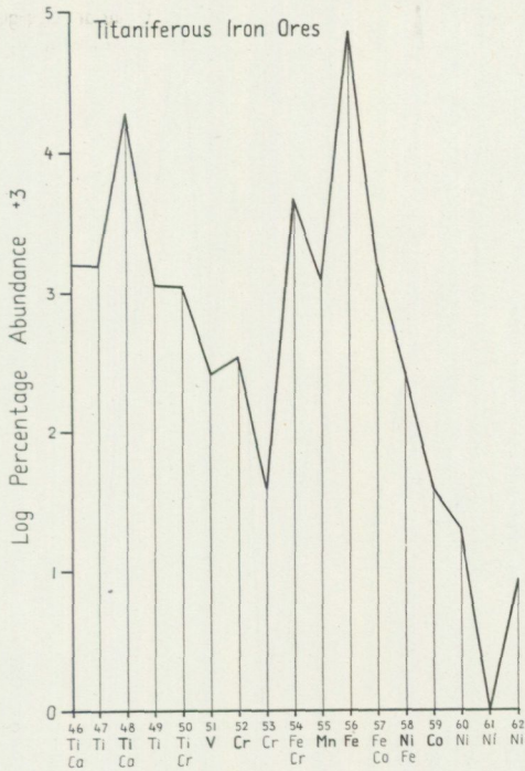
Fig. 23. Diagram of the percentage abundance of the ferride isotopes with mass-numbers 46—62 in titaniferous iron ores.
