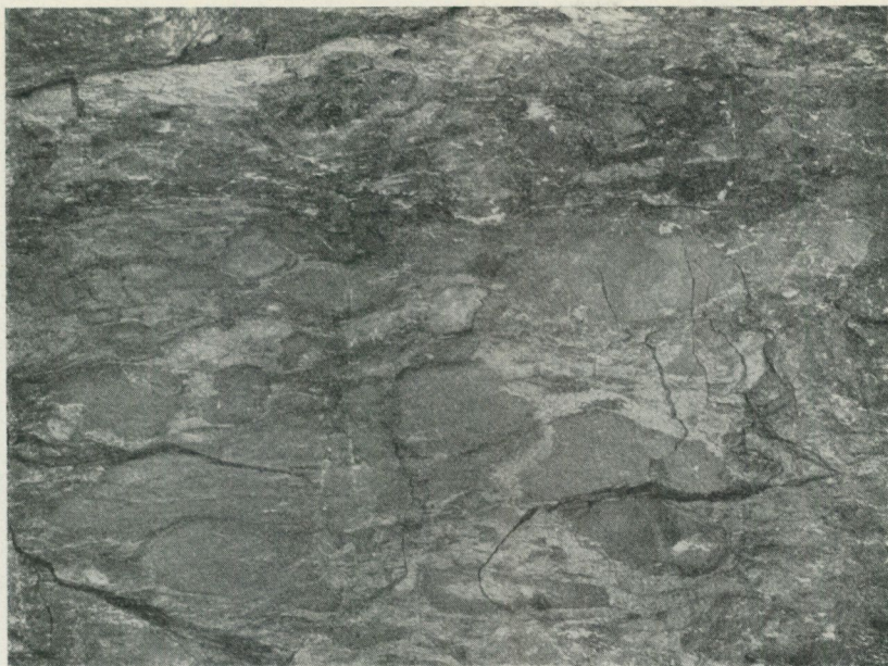
Fig. 8. Quartz-porphry conglomerate, sericitized and richly impregnated with pyrite replacing the groundmass of the conglomerate. Roof of a drift at 150 m level in the Mensträsk mine. Scale 1 : 10.
