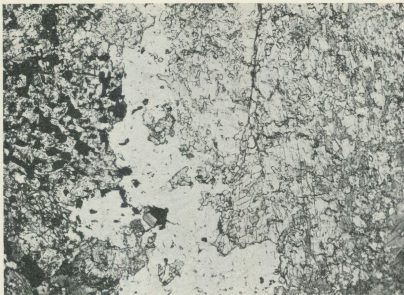
Fig. 13. Complex skarn. Pyroxene with hornblende relics to the right, anorthite in the middle, epidote and sulphides to the left in the photograph. Ord. light. \times 25 .
