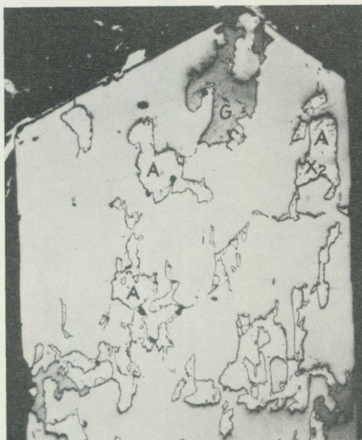
Fig. 1. Big crystal of arsenopyrite, partly replaced by galena (G), and altaite (A). In the upper right altaite area a band of mineral X 2 . Green filter. Oil immersion. × 300.
