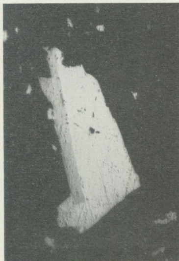
Fig. 6. Altaite (white) with mineral X_1 (light grey). Green filter. Oil immersion. \times 400 .
