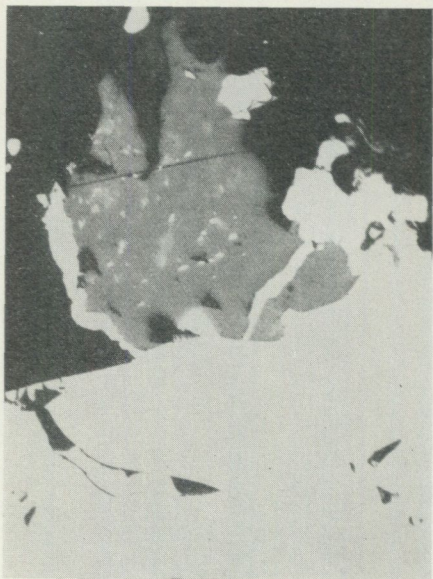
Fig. 3. Sphalerite (grey) with small blebs of chalcopyrite is replaced by tetrahedrite (white). Green filter. Oil immersion. \times 400 .
