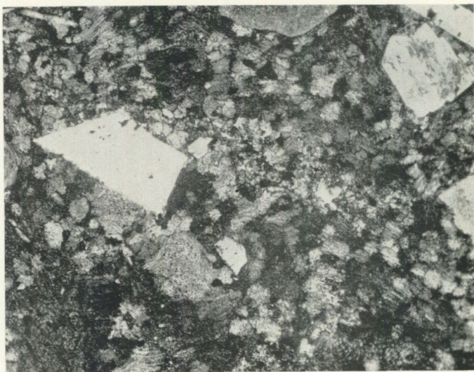
Fig. 12. The same as fig. 11, crossed nic. The devitrification has proceeded far, and between crossed nic. the eutaxitic structure is no more visible but is replaced by a maculose appearance.
