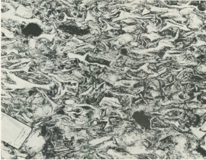
Fig. 1. Ignimbrite from Te Miro, near Cambridge, North Island of New Zealand. 30 x. To the lower left small phenocryst of oligoclase. The welded groundmass is porous and built up of bent and Y-shaped glass fragments some of which are vesicular.
