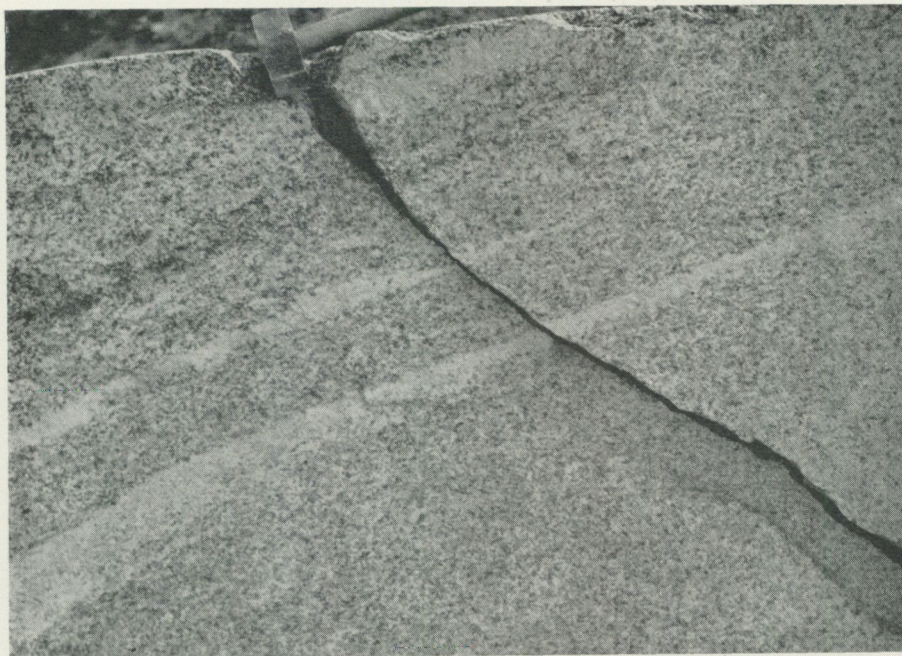
Fig. 20. Bands of felspar and quartz in primorogenic basic granite (Uppsala granite). Road-cutting 4.5 km W.N.W. of Bergsbrunna stn.
