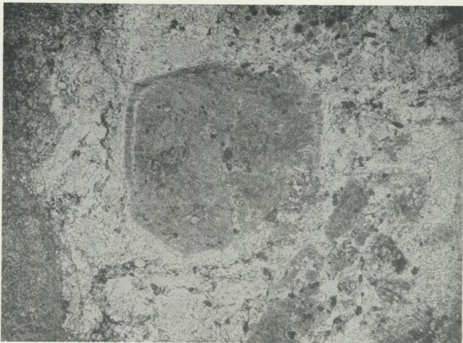
Fig. 9. Plagioclase phenocryst in plagioclase-porphyrite. Thin section magnified 25 \times . 1.5 km E.N.E. of Läby church.
