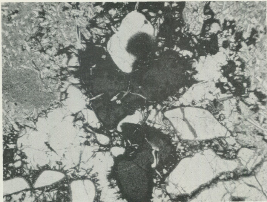
Fig. 12. Xenolith composed of secondary glass and serpentine in devitrified lava. Thin section magnified 24\times . Photo N. Sundberg 1955.
