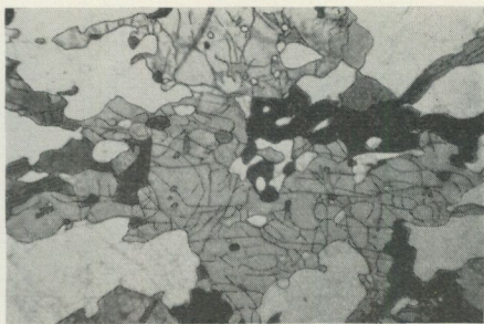
Fig. 11. Penetrating hypersthene in norite. Kramsta massif. 1 nic., magnification 14 ×. Photos by P. H. Lundegårdh.
