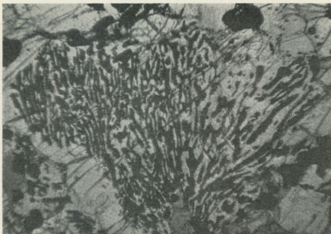
Fig. 15. Fingering oxidic ore inclusions in clinopyroxene. Norite from the neighbourhood of Tallåsen, Northern Helsingland (no 6 in Fig. 1). 1 nic., magnification 65 \times . Photo by P. H. Lundegårdh.
