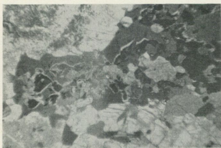
Fig. 10. Cataclastic texture in noritic gabbro: Granulated and uralitized pyroxene with titaniferous iron ore, surrounded by non-affected plagioclase. Gartsbo (Fig. 3). 1 nic., magnification 14 ×.
