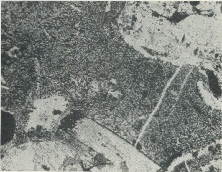
Fig. 5. Porphyry fragments in a younger sediment. Amygdales and plagioclase phenocryst in a groundmass of plagioclase lathes and iron ore margarites. — One nicol. Magnification approx. 115.
