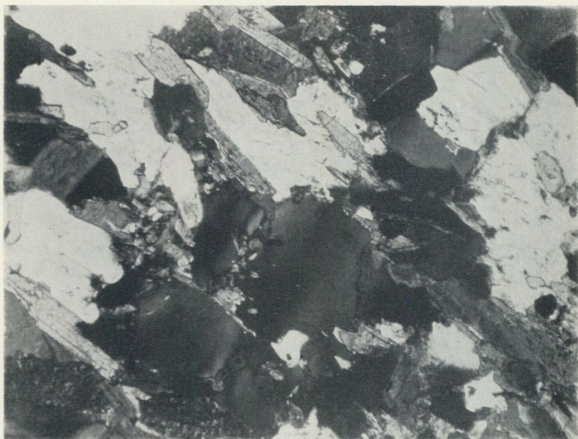
Fig. 5. Skapolit-biotit-hornblände-fels, borrhål 58118, 58.30 m. Slipprov, + nic., 75 \times . Scapolite-biotite-hornblende-fels, drill-hole 58118, 58.30 m. Thin section, + nic., 75 \times .
