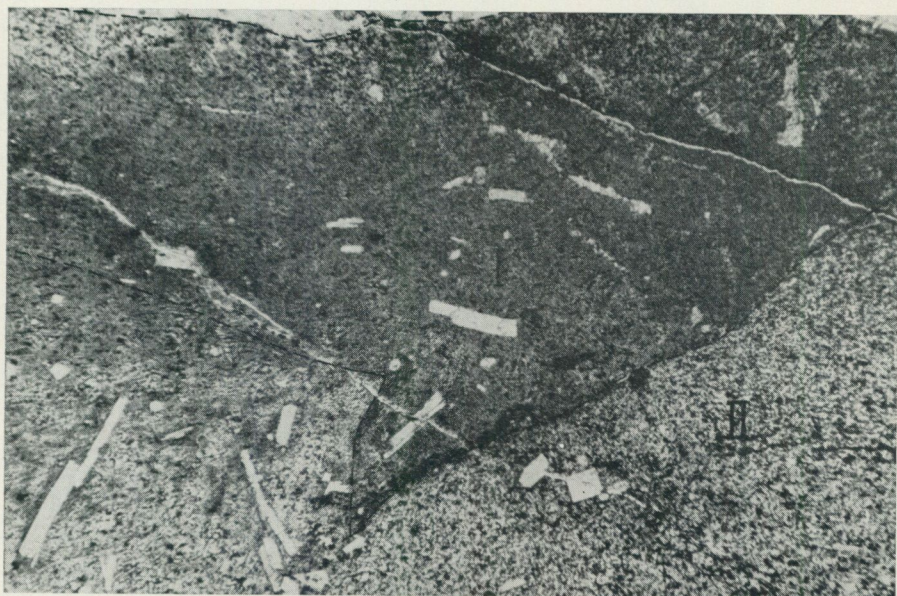
Fig. 77. Dolerite dike with two generations of intrusion. Brattön 338.585. Ord. light. 30 x.
