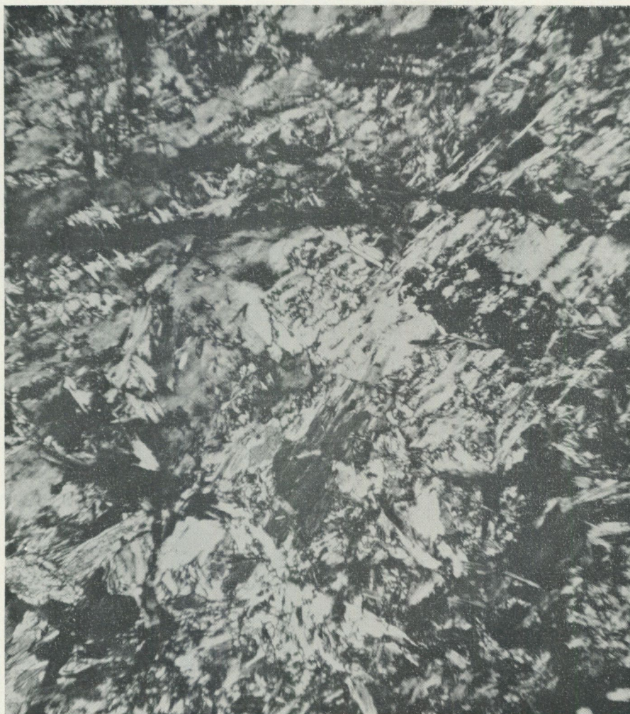
Fig. 13. Mesh of antigorite, penninite, and talc in peridotite. Aröd 367.668. Nic. +. 25×.
