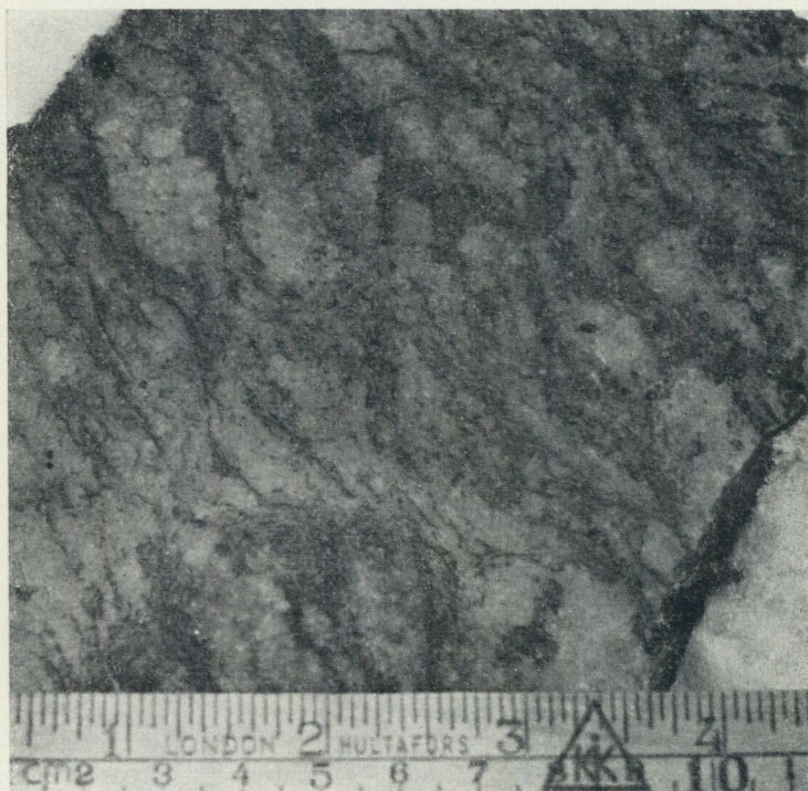
Fig. 51. Granitic augen-gneiss. Polished specimen. Häller 176.794.
