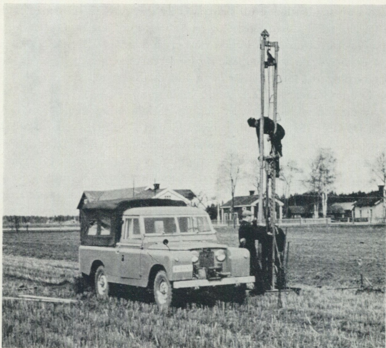
Fig. 1. Foliekärnborren under arbete. Hela utrustningen transporteras med en jeep. The boring device in working position. The whole equipment is transported by a jeep.
