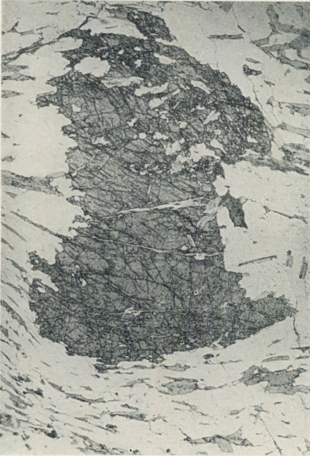
Fig. 11. Porphyroblast of gahnite in quartz-mica schist, Skvasselbo group. Microphoto. of thin section, ord. light, x 11. E. Welin, photo.
