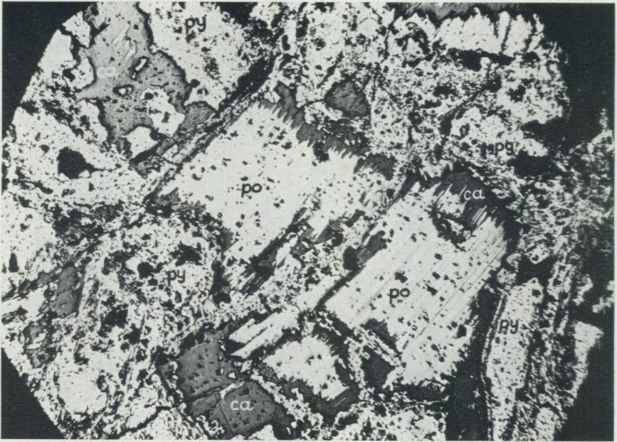
Fig. 16. Alteration of pyrrhotite to pyrite. The pyrrhotite (po) appears as light crystals with prominent cleavages, surrounded by pyrite (py) and calcite (ca). Dh 62014 47.3 m. Polished specimen. \times 20 .
