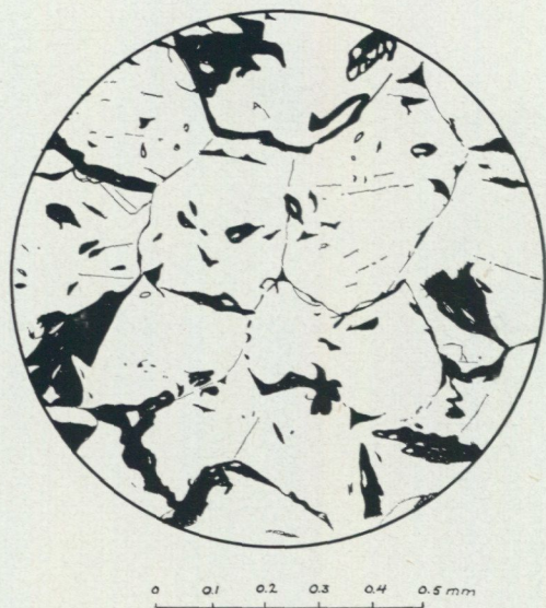
Fig. 14. Magnetite ore with magnetite (white) and serpentine (black). Drawing from polished specimen. Dh 62014 47.3 m.
