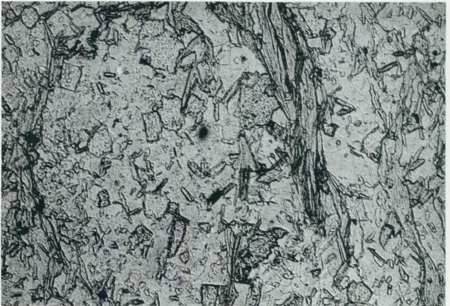
Fig. 5. Sericite-chlorite schist with anhydrite (rectangular grains with strong relief), Kristineberg mine, 490 metres level, 30 metres S of fixed point 29. Without analyser. 35x.
