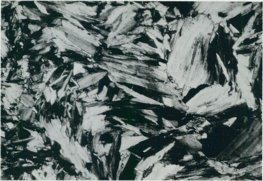
Fig. 7. Chloritite. The older schistosity cut by a younger cleavage. The style is more brittle than in fig. 6. In the vicinity of the Kimheden ore. Crossed nicols. 35x.
