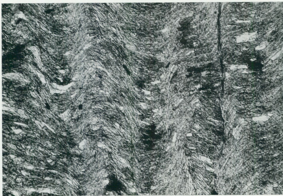
Fig. 11. Folded phyllite. The folding of the bedding fissility is the incipient stage of the formation of a younger cleavage. Shore of the Storforsen rapid. Without analysator. 175x.
