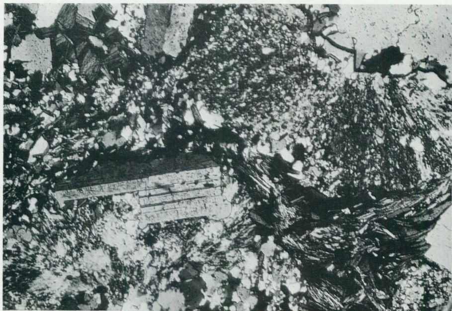
Fig. 4. Keratophyre with spherulites. In the vicinity of Kimheden ore. Crossed nicols. 35x.
