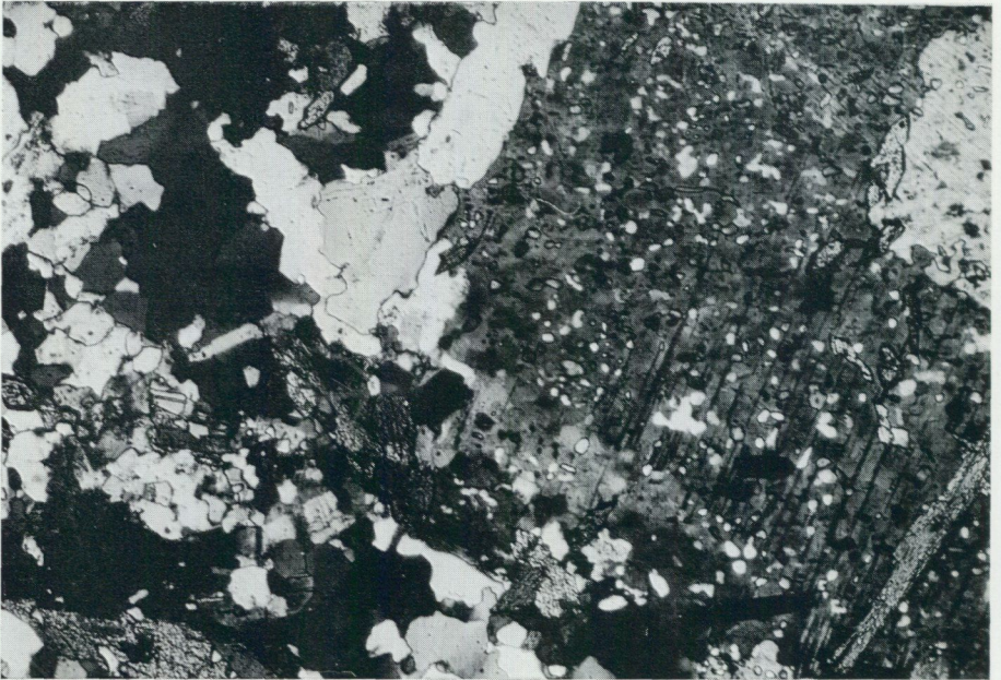
Fig. 3. Gneiss with plagioclase porphyroblasts in a fine-grained matrix. Exposure outside the map area, E of Viterliden. Crossed nicols. 35x.
