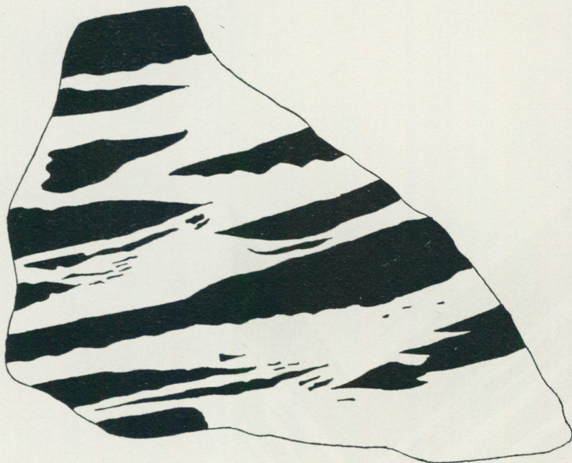
Fig. 4. Apatite rock (white) and pure magnetite ore (black); specimen from Tuolluvaara. Slightly reduced from natural size.
