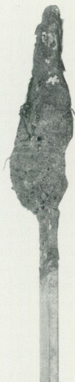
Fig. 1. A piece of sherardized iron that has been in soil for two years. A crust hard as stone is formed on that part which has been in the soil. The crust is formed from sand cemented with calcite and other salts, amongst others, large amounts of phosphate. The colour is dark brown because of a high humus content. Half natural size.
