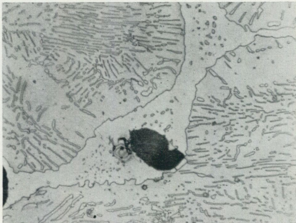
Fig. 5. Fines from Grängesberg reduced at 1050° C. Pearlitic matrix. Steadite (mottled light grey band) and a silicate inclusion (dark grey). 750 ×.
