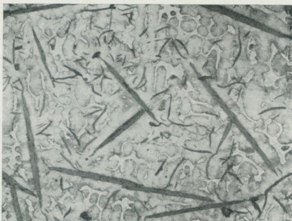
Fig. 6. Lake ore reduced at 1200° C. Pearlitic matrix with steadite. Graphite flakes (dark grey). 150 ×.
