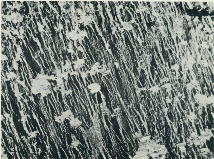
Figure 4. Vein perthite and patch perthite in the same grain. 2 nic., \times 50 . (Hornblende granite: T 15/Nr 137.)
