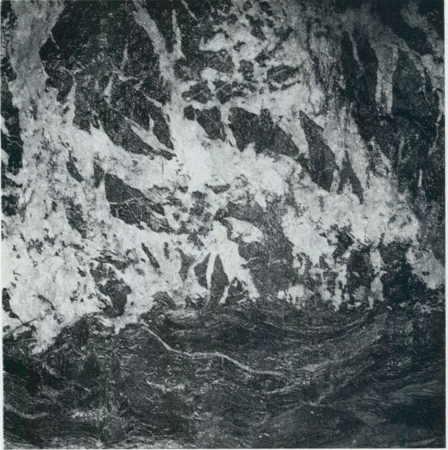
Fig. 13. Photo of the quartz-tourmaline vein in Stope 64, S-side of the roof, cf. fig. 12. Scale about 1:20.
