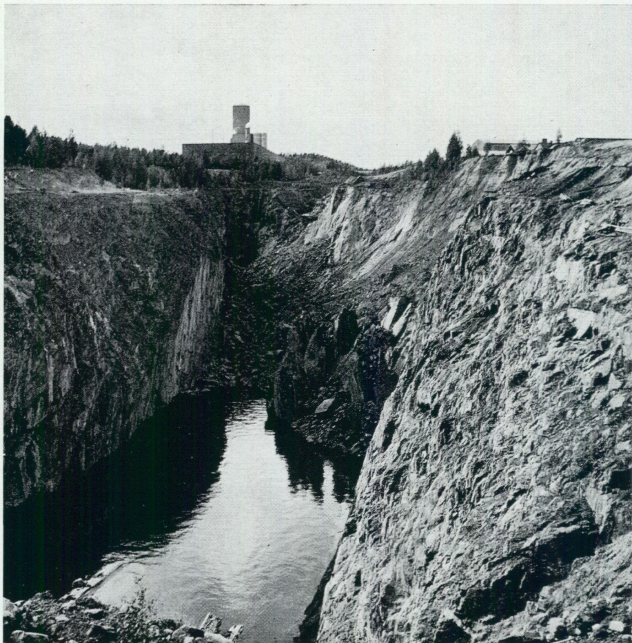
Fig. 21. View looking west from the east end of the Boliden open pit. Note the steeply dipping hanging wall on the left side, along which the a-d-arsenopyrite ore lense (Fig. 22) lay. There the altered rocks extended for only a few metres outwards from the ore contact before being followed by fresh quartz keratophyre. This wall was very strong and stood practically undisturbed down to the bottom of the pit at the 90 m level. Around the fault line crossing the ore to the right in the photo there have been subsidences for a long time, cf. chapter 10. In the distance one can see a glimpse of the dressing plant. The section shown in Fig. 23 cuts the water-filled part of the pit. Photo by E. Grip, 1969.
