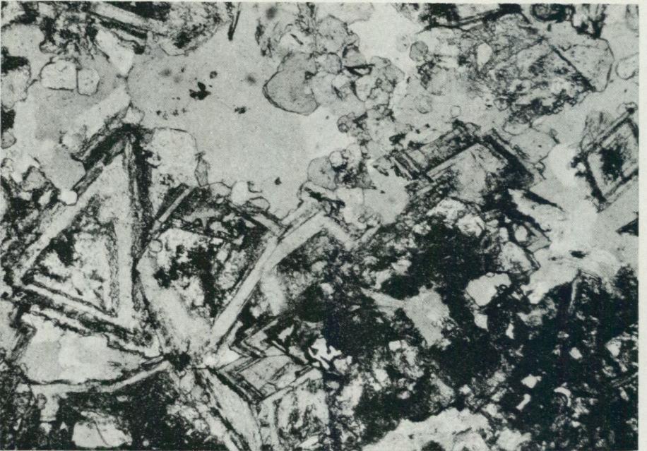
Fig. 2. Zoned carbonate in limestone. Nicols parallel. Magn. 60 x. Sample 27/67 Lauttakoski.
