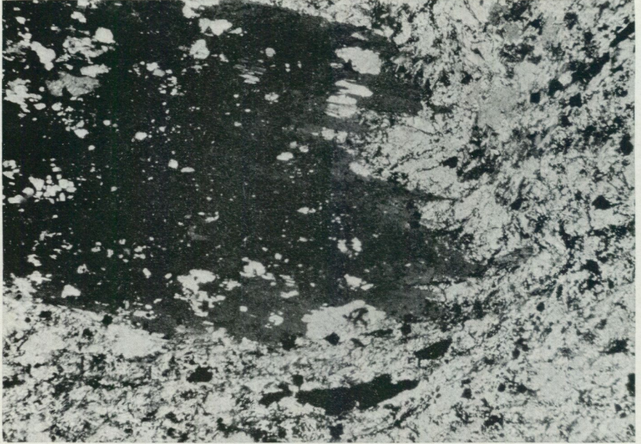
Fig. 15. Carbonatized and steatitized amphibole in soapstone. Nicols crossed. Magn. 37 x. Sample 19/69 Lauttakoski.
