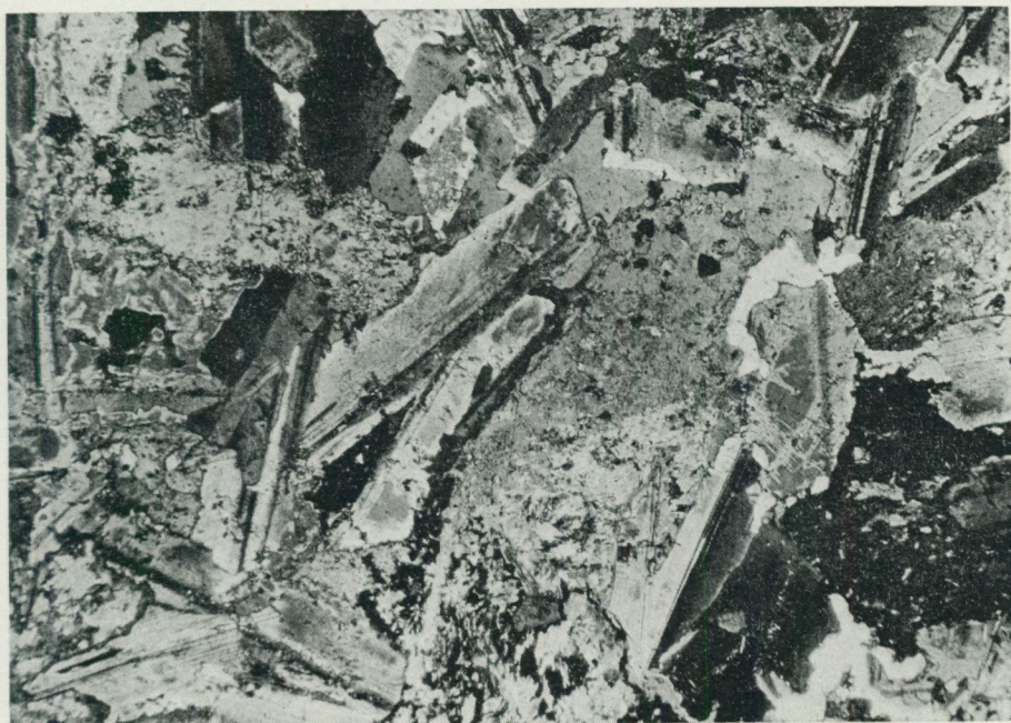
Fig. 6. Intersertal texture in meta-diabase. Nicols crossed. Magn. 30 x. Sample 40/69 Lauttakoski.
