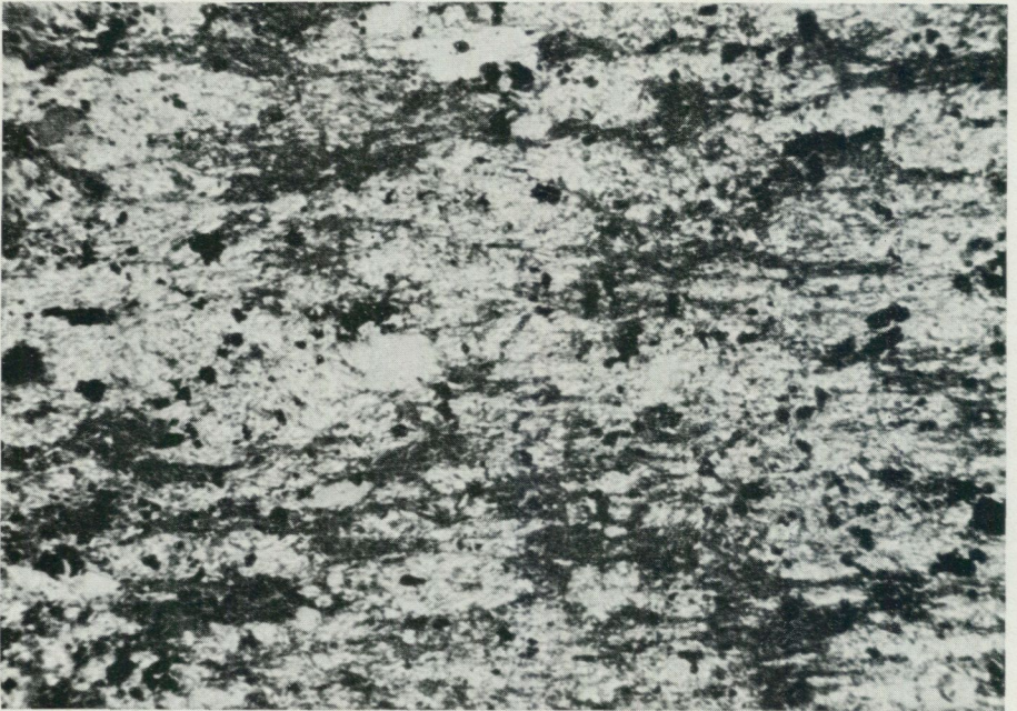
Fig. 16. Schistose soapstone. Long stretched (dark) aggregates of chlorite. Nicols crossed. Magn. 37 x. Sample 1/66 Lauttakoski.
