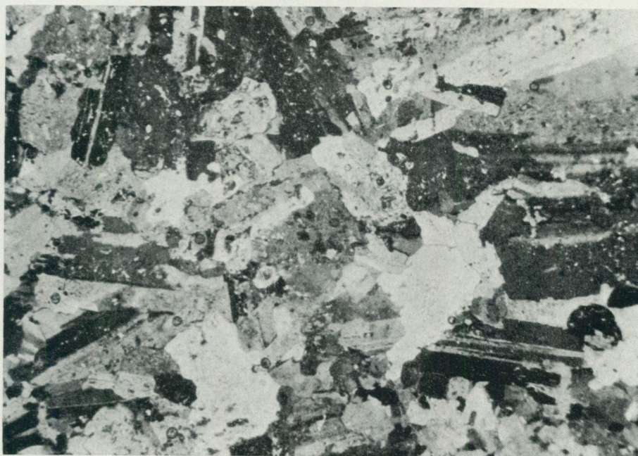
Fig. 11 Intersertal texture in carbonate-rich albitite; albite crystals practically unaltered with interstitial carbonate. Nicols crossed. Magn. 37 x. Sample 16/67 Lauttakoski.
