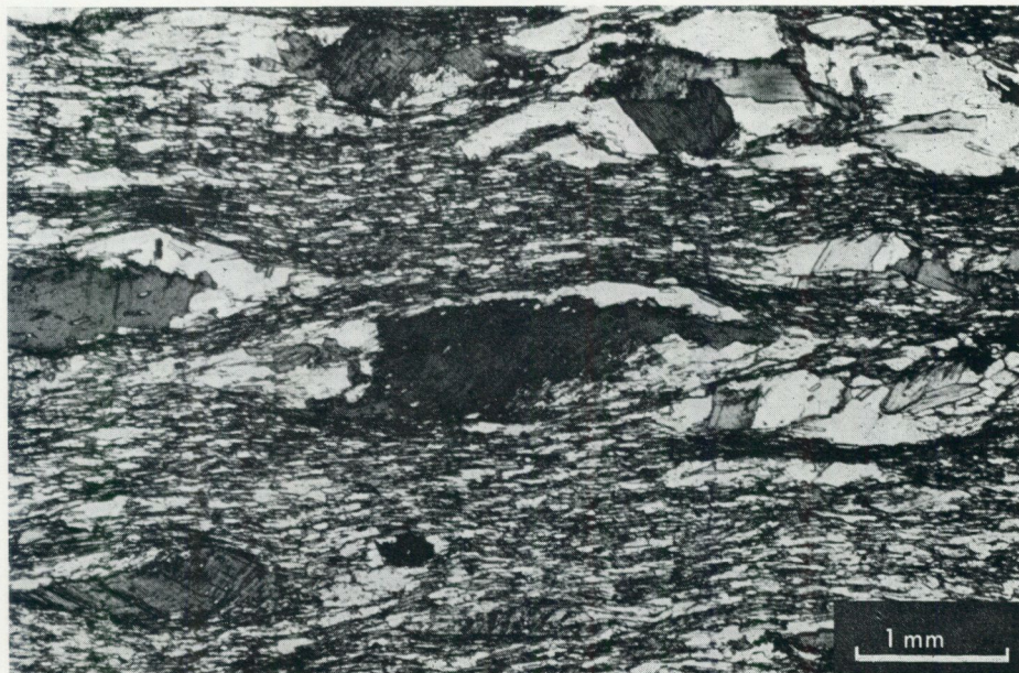
Fig. II-13. Slaty cleavage in the eastern part of the phyllite belt, curving around biotite porphyroblasts with straight or slightly S-shaped inclusions. S_1 is continuous with S_2 .
