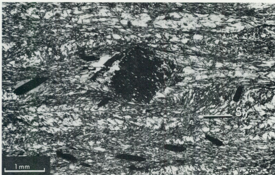
Fig. II-12. Interkinematic biotite porphyroblast with planar S_1 fabric, interpreted as S_1 . The surrounding crenulation cleavage, S_2 , curves around the crystal. Ilmenite crystals are oriented parallel to S_1 .
