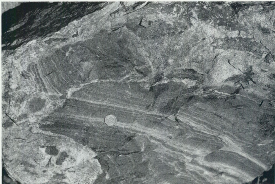
Fig. 3. Apatite-banded magnetite ore surrounded and partly brecciated by apatite. Nukutus.
