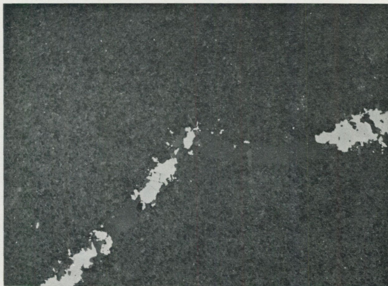
Fig. 13. Chalcopyrite in a pebble from sample No. 5. Test-pit 1. Polished section. Ord. light. \times 50 .
