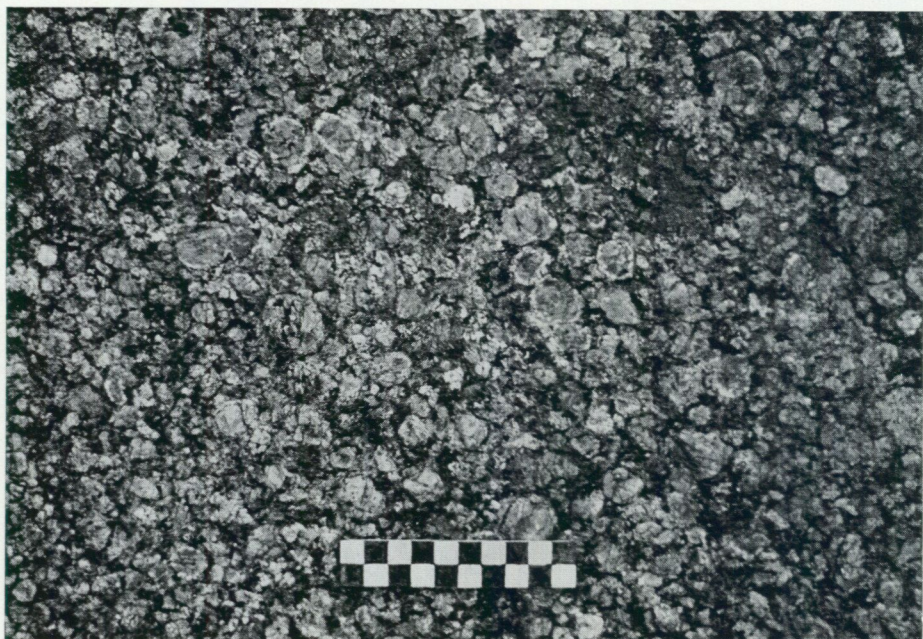
Fig. 24. Yasjö granitoid with sub-rounded potash feldspar megacrysts, frequently mantled by plagioclase. Yasjön.
