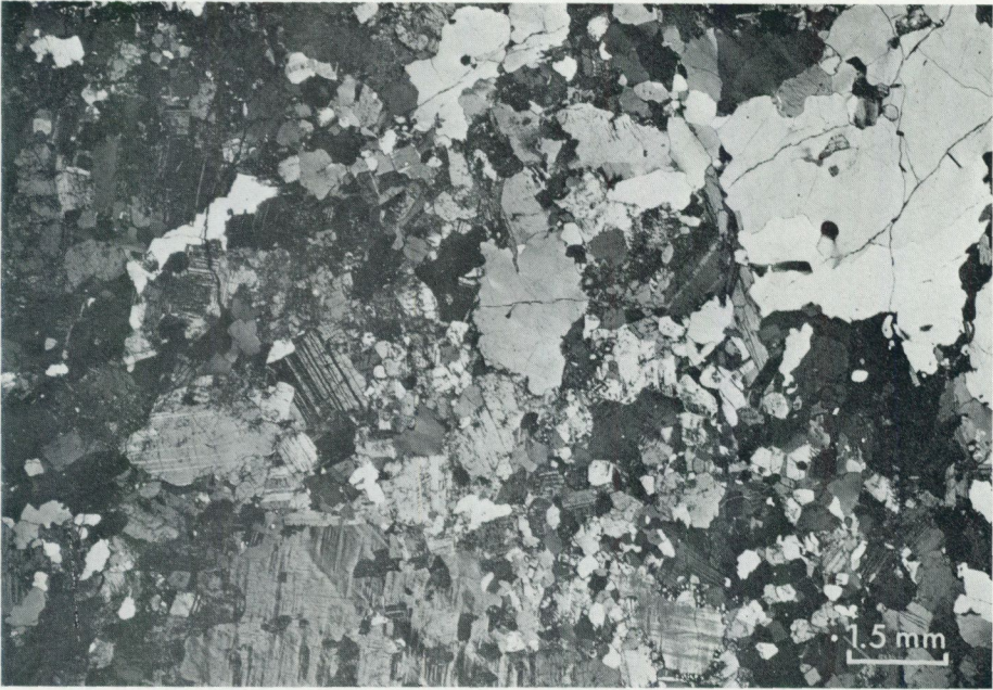
Fig. 8. Older granitoid of tonalitic composition. Deformed plagioclase megacryst (left below). 2 nic. 1.7 km ENE of Tving village (WC 303417).
