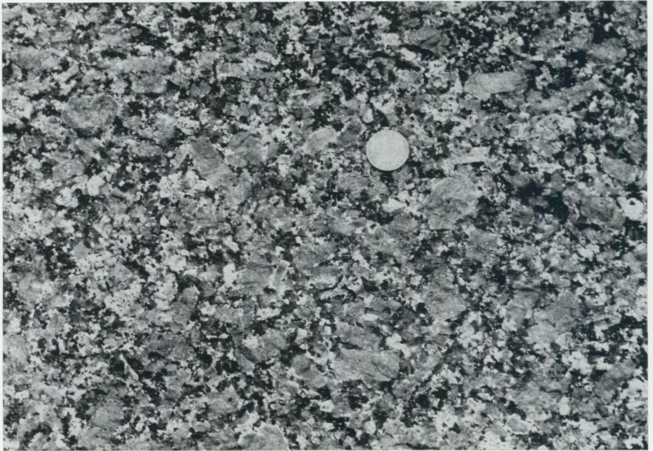
Fig. 20. Eringsboda granitoid with sub-rectangular potash feldspar megacrysts. Some megacrysts are plagioclase (whitish) mantled (below centre). Guttamåla.
