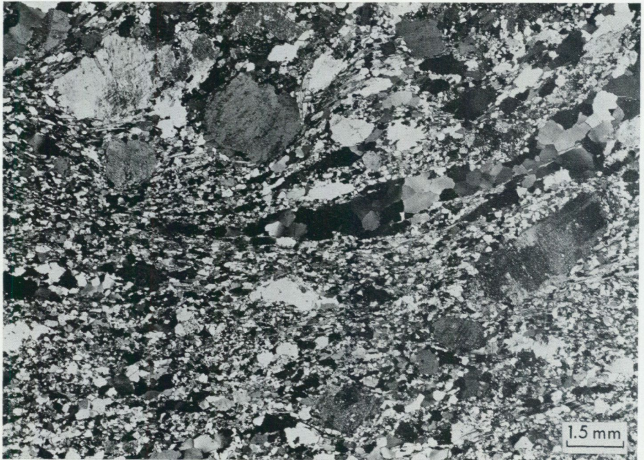
Fig. 18. Deformed Younger granitoid with lenses of quartz and feldspar porphyroclasts in a fine-grained matrix. 2 nic. S of Flymen village.
