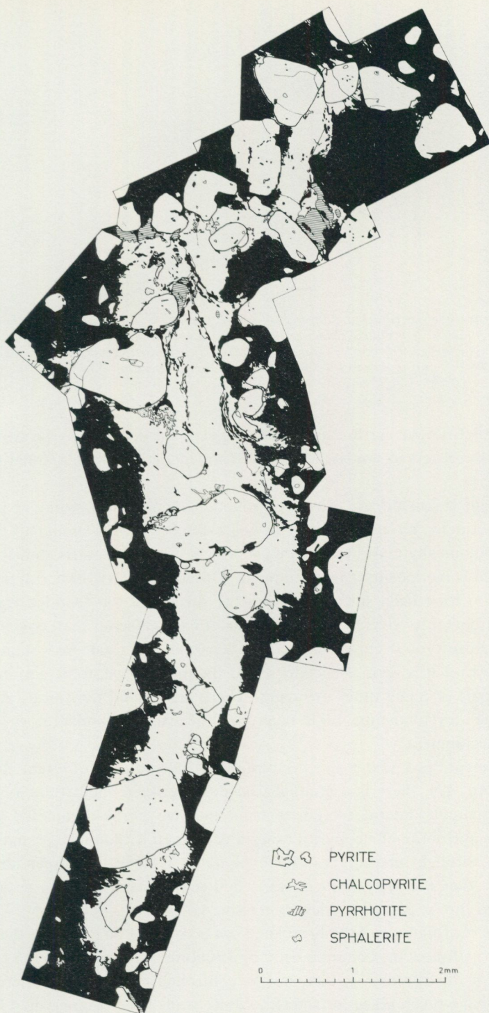
Fig. 50. Detail of breccia ore containing much chalcopyrite and a large quantity of rounded pyrite individuals. Small sphalerite areas visible near pyrite grains. The sample is unusually low in pyrrhotite. Host rock—tuffite. Drawing after microphoto mozaic, M. Bergman.
