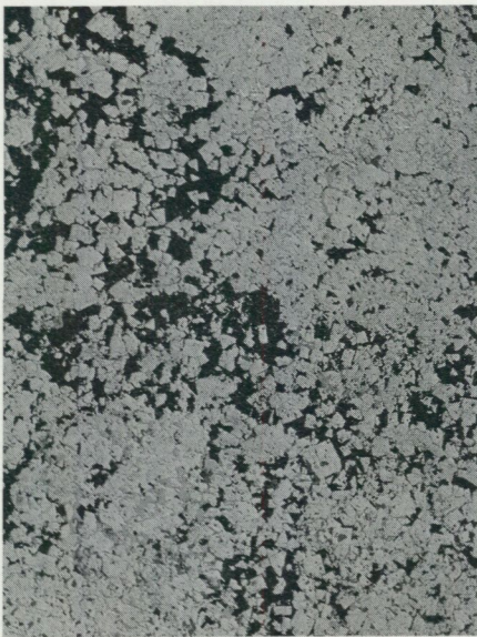
b) Pyrite-sphalerite-chalcopryrite ore. Patch-wise fine-grained island-like aggregates with irregular outlines "floating" in areas with more gangue and somewhat coarser pyrite. No banding visible on the scale of the polished section.
