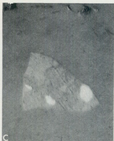
Fig. 35. Fahlore with inclusions of hessite. a) Hessite (single and with droplets of gold) and chalcopyrite (single and with one arsenopyrite crystal). 125 X. b) Hessite containing three droplets of gold seen under ordinary light in oil immersion. Detail from Fig. 33 a. 960 X. c) The hessite grain, consisting of several individuals, demonstrates the anisotropy of the mineral under crossed nicols. 960 X.
