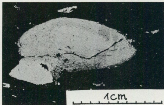
Fig. 9. Zoned and deformed pyrite nodule, consisting of individuals of 10—50 \mu . Darker shade in outer zone is due to minute interstitial particles. Dark band across right part is due to etching.
