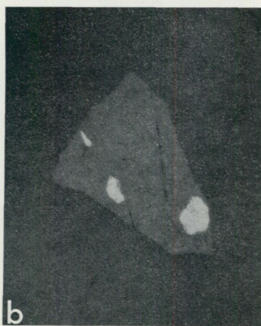
Fig. 35. Fahlore with inclusions of hessite. a) Hessite (single and with droplets of gold) and chalcopyrite (single and with one arsenopyrite crystal). 125 X. b) Hessite containing three droplets of gold seen under ordinary light in oil immersion. Detail from Fig. 33 a. 960 X. c) The hessite grain, consisting of several individuals, demonstrates the anisotropy of the mineral under crossed nicols. 960 X.
