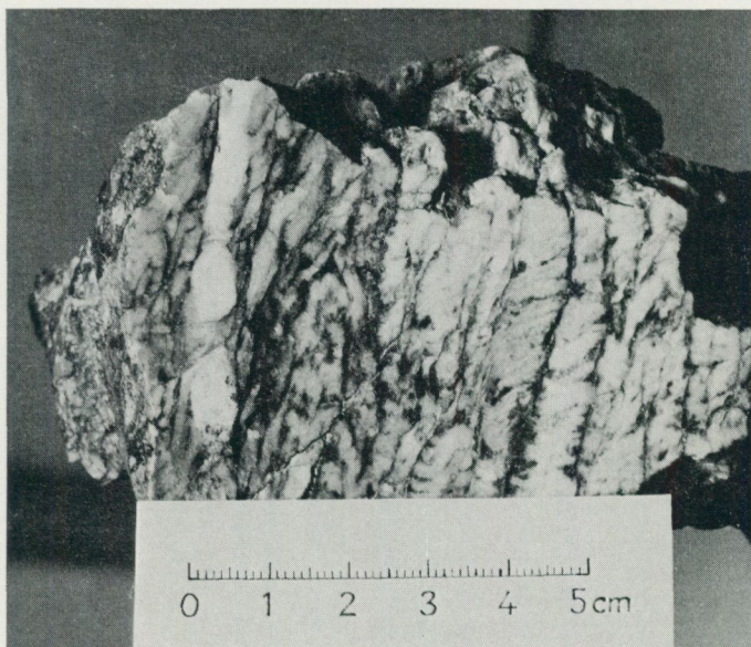
Fig. 58. Shattered quartz-keratophyre with very fine-grained, vein-like impregnations of chalcopyrite.
