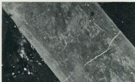
Fig. 28. Irregular zoning in arsenopyrite. Crossed nicols. 60 X.
