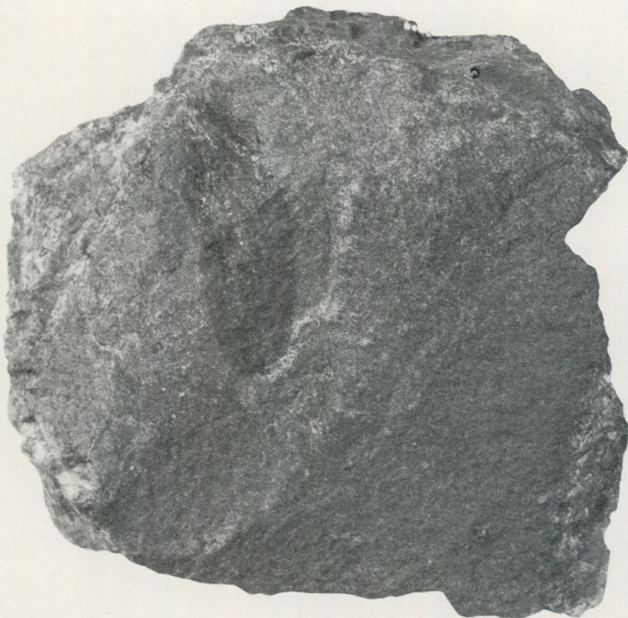
Fig. 18. Pebble of P-poor magnetite ore in a fragment of P-rich magnetite ore from the hanging wall porphyry. Luossavaara.
