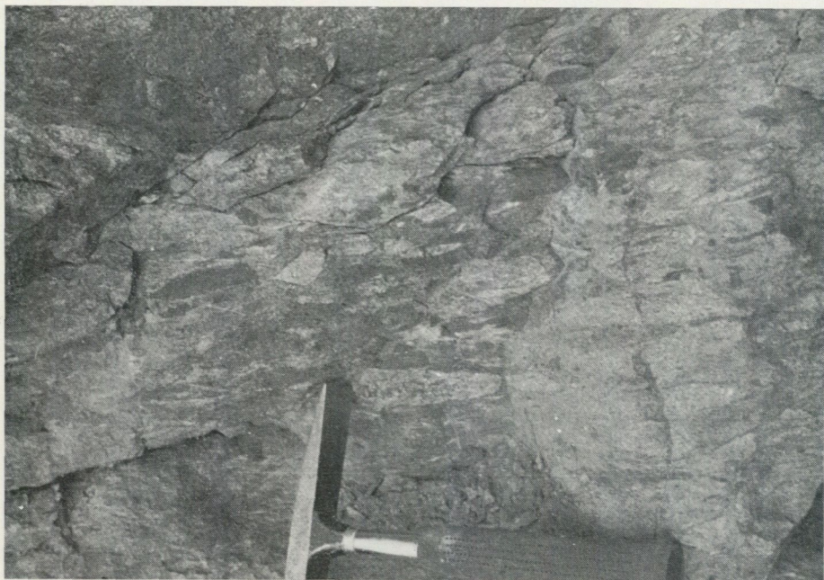
Fig. 11. Polymictic fragments in the quartz-bearing porphyry, near to the ore contact. Rektorn.
