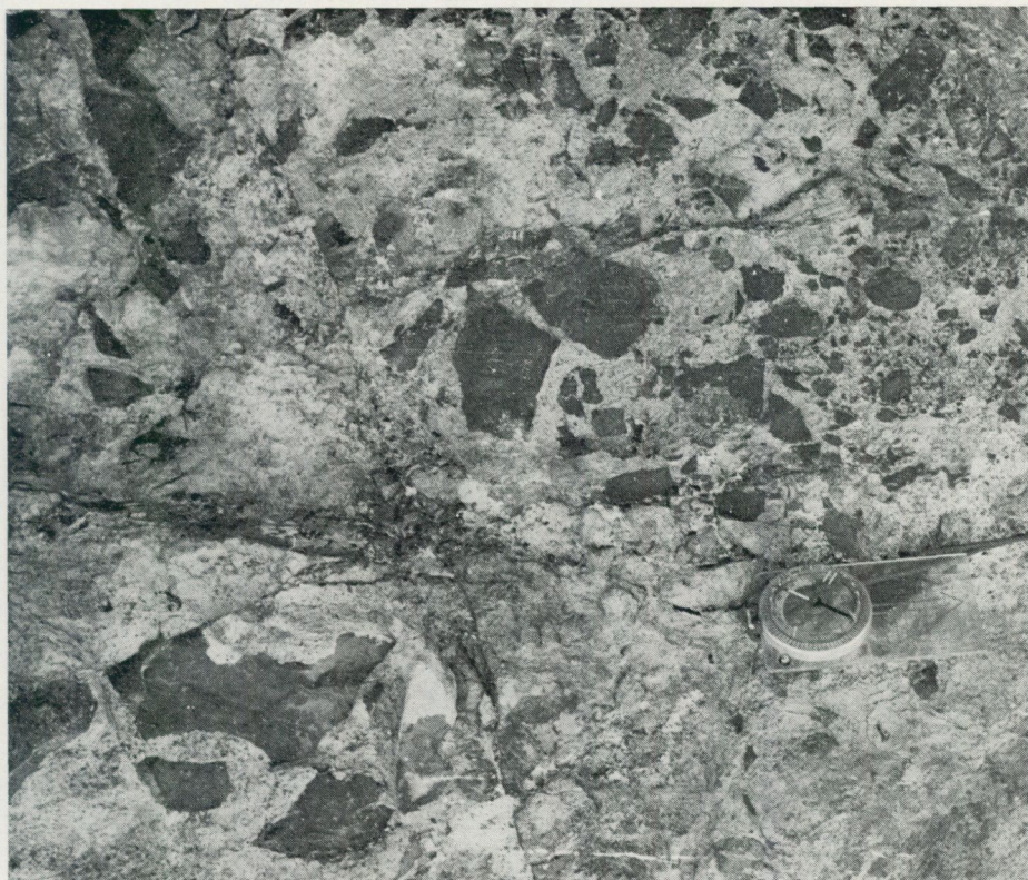
Fig. 54. Fragments of hematite ore in apatite. Henry.
