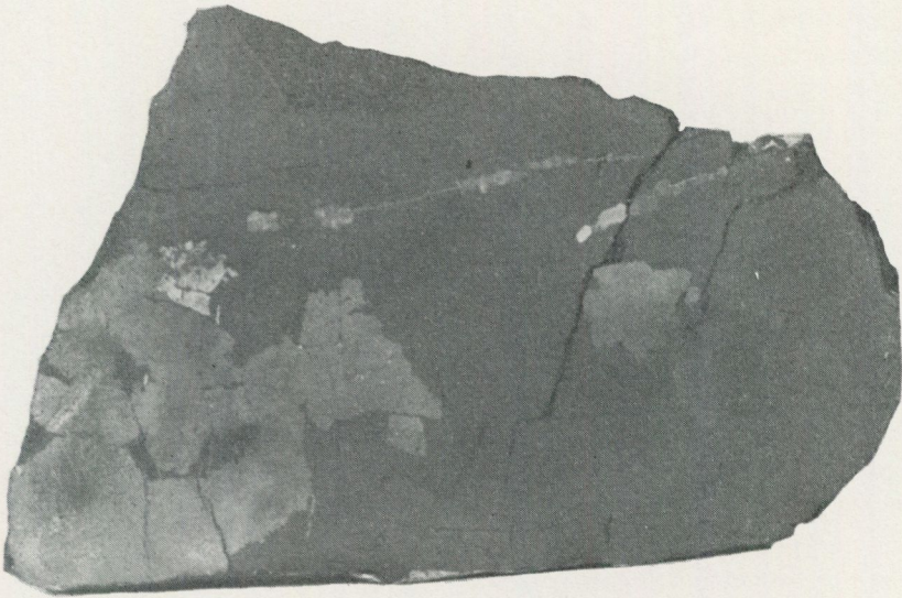
Fig. 26. Hematite (grey white) in magnetite ore. Tuolluvaara. Photo B. Rönberg.
