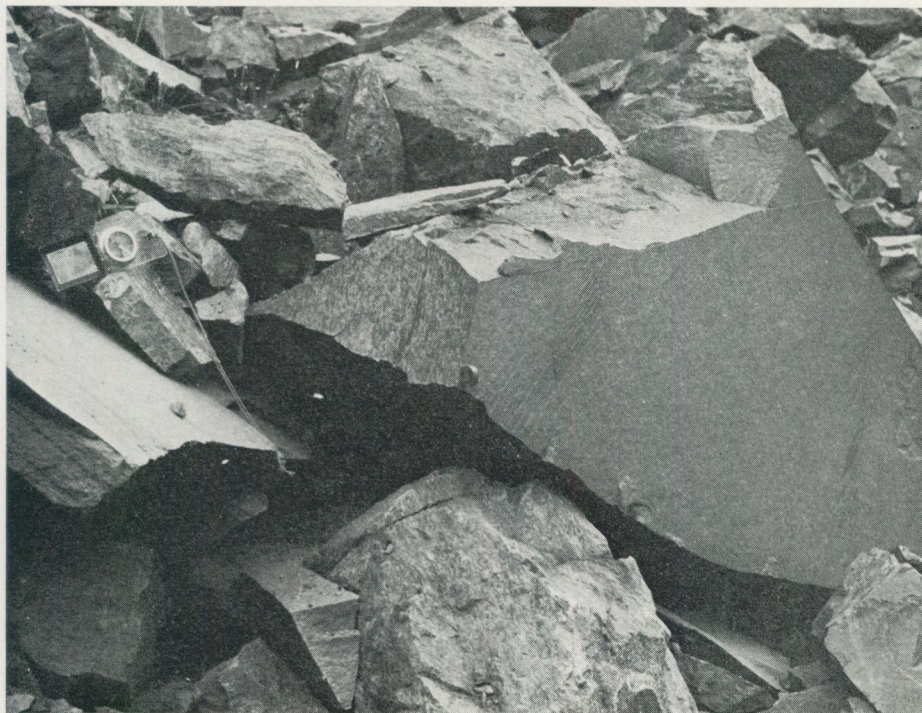
Fig. 28. Plane schistosity in magnetite ore. Rektorn.
