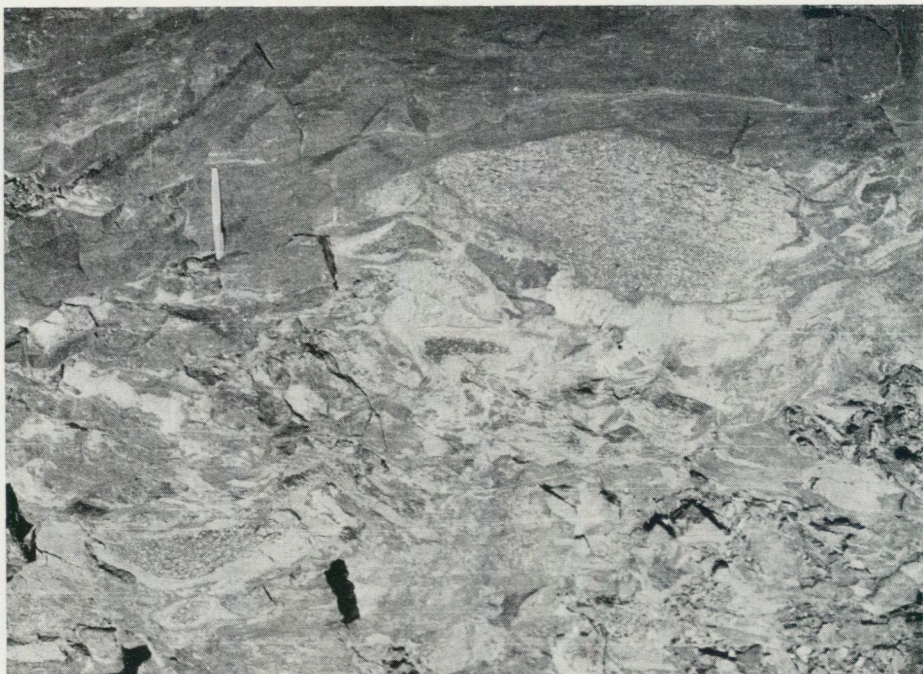
Fig. 53. The apatite-banded ore resting on a weathering breccia. Rektorn.
