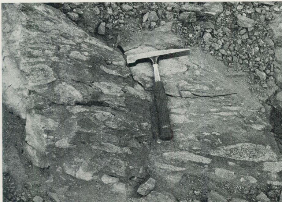
Fig. 10. Fragments of rocks and iron ores in a matrix essentially composed of apatite and magnetite.
